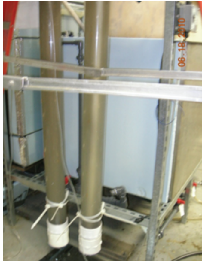
Figure 17. Water columns (2.4 meters) containing turbid water used to evaluate egg adhesion.
