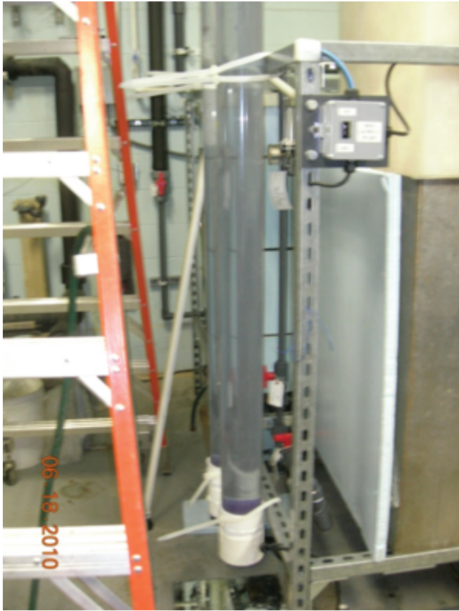
Figure 16. Water columns (4.0 meters) used to determine vertical distribution of free embryos and their ability to fill their swim bladders.
