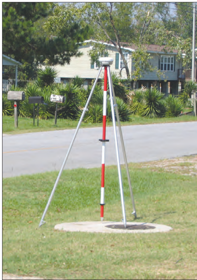
Figure 5. Typical global positioning system equipment used to survey storm-tide elevation after Hurricane Irene (photograph by Jonathan J. Graham, USGS).
