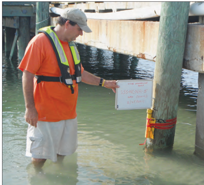
Figure 2. USGS employee deploys storm-tide sensor at Wrightsville Beach, North Carolina, August 25, 2011 (photo by Frank Melendez, USGS).
