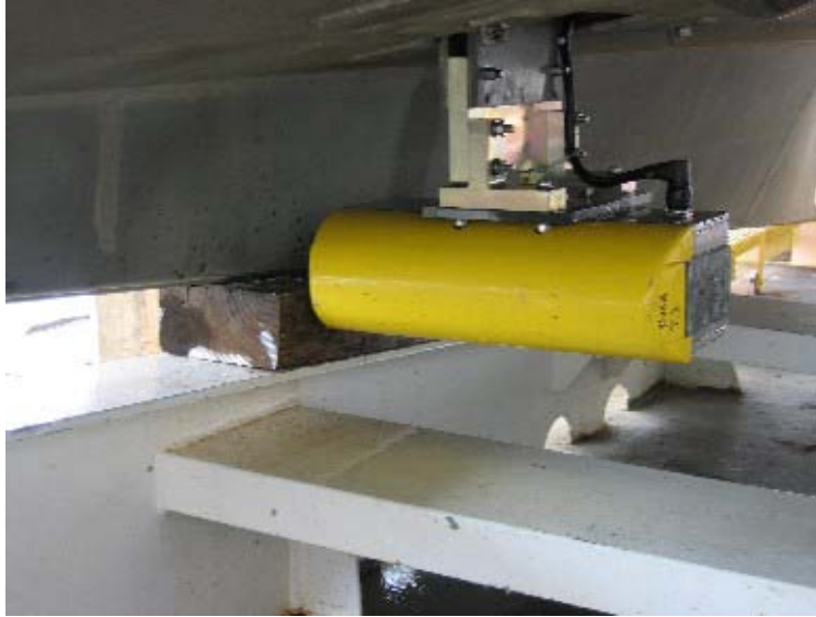
Figure A-5. 8125 Housing on Launch 3101
