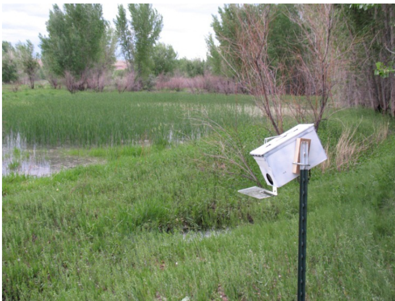
An acoustic monitoring station at Ouray NWR. Anabat ultrasonic bat detectors were fitted inside metal cases and affixed to steel posts. Photo by Laura E. Ellison.
