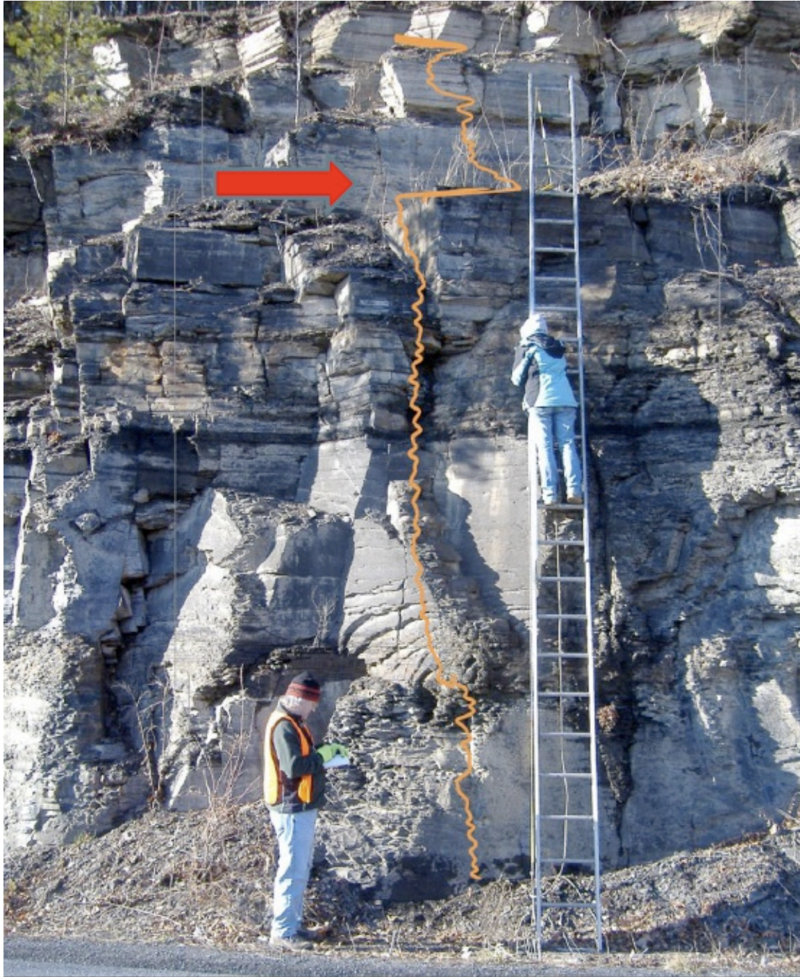
Figure 26. The synthetic gamma ray log of the Millboro Shale that was obtained from the outcrop at stop 3 in February 2011 is overlain on the exposure itself. The arrow is at the horizon of the major observed kick in counts per second and probably marks the location of the zone of highest organic content in this exposure. John Haynes and James Madison University student Sharon Porter are shown in photo. Photo: Richard Lambert, VSS.
