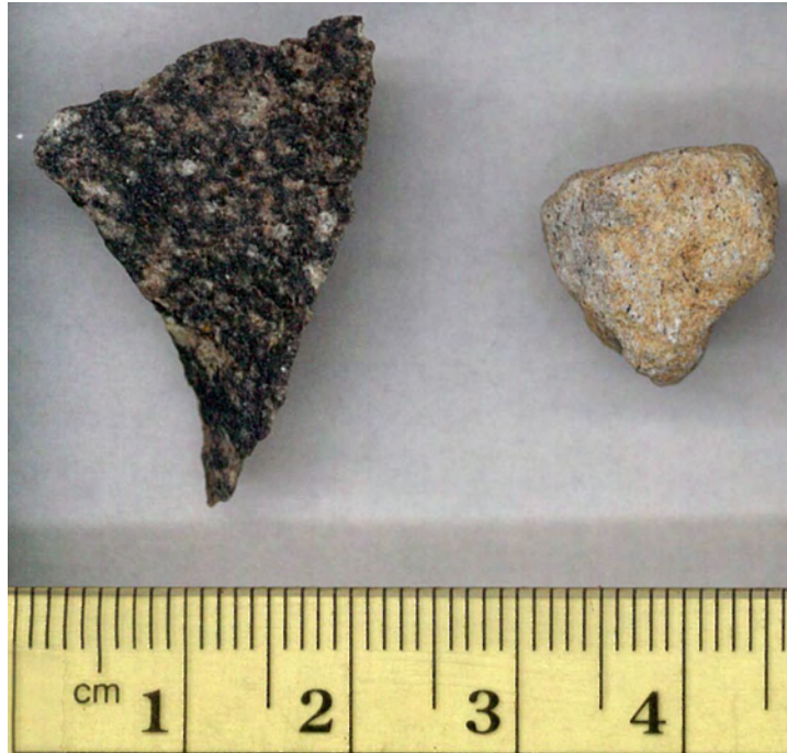
Figure 7. Photograph showing examples of grains with fractured and broken surfaces (left) and original surfaces (right).
