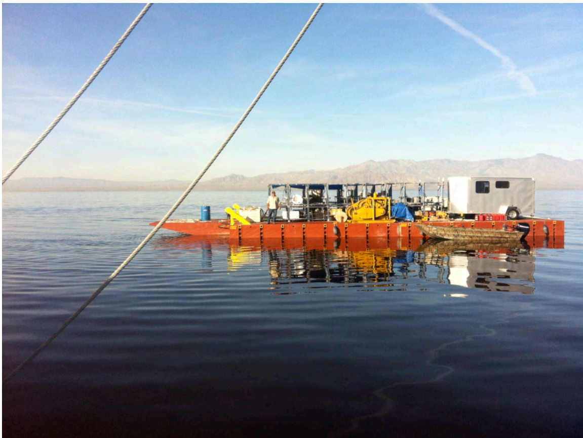
Figure 19. Photograph of barge constructed on site to accommodate the marine part of SSIP. The white trailer on the right housed the acquisition computers. OBSs were stored in the (empty) racks in the central part of the barge. The gold-colored unit in the center was the anchor winch. The compressor for the air guns was located on the other side of the barge, out of view.
