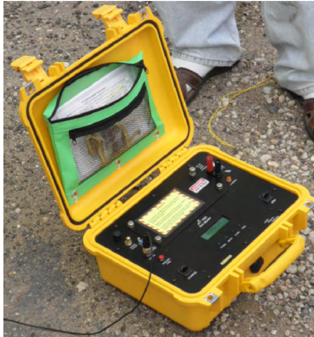
Figure 13. Photograph of the shooting system built for SSIP by retired electronic engineer and explosives handler, Edward Jensen. GPS antenna (out of the photograph to the left) is attached to the system by small black cable shown. Shot wire (yellow wire in upper right) is attached to the red and black terminals on the right side of the box. The shooting system releases a stored charge into the shot wire on the exact minute mark following arming of the system.
