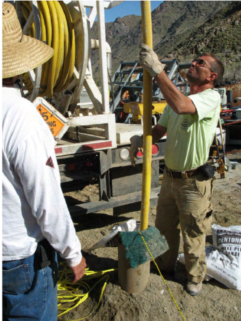
Figure 8. Photograph of U.S. Geological Survey personnel loading blasting agent into shot hole 60000 using the pump truck. The detonating cord (yellow, lower-right corner of photograph) and booster assembly has been lowered to the bottom of the hole. The plastic bentonite bags and green “horse-hair” pad around the top of the steel casing prevents chafing of both the hose and the detonating cord against the coarsely cut metal.
