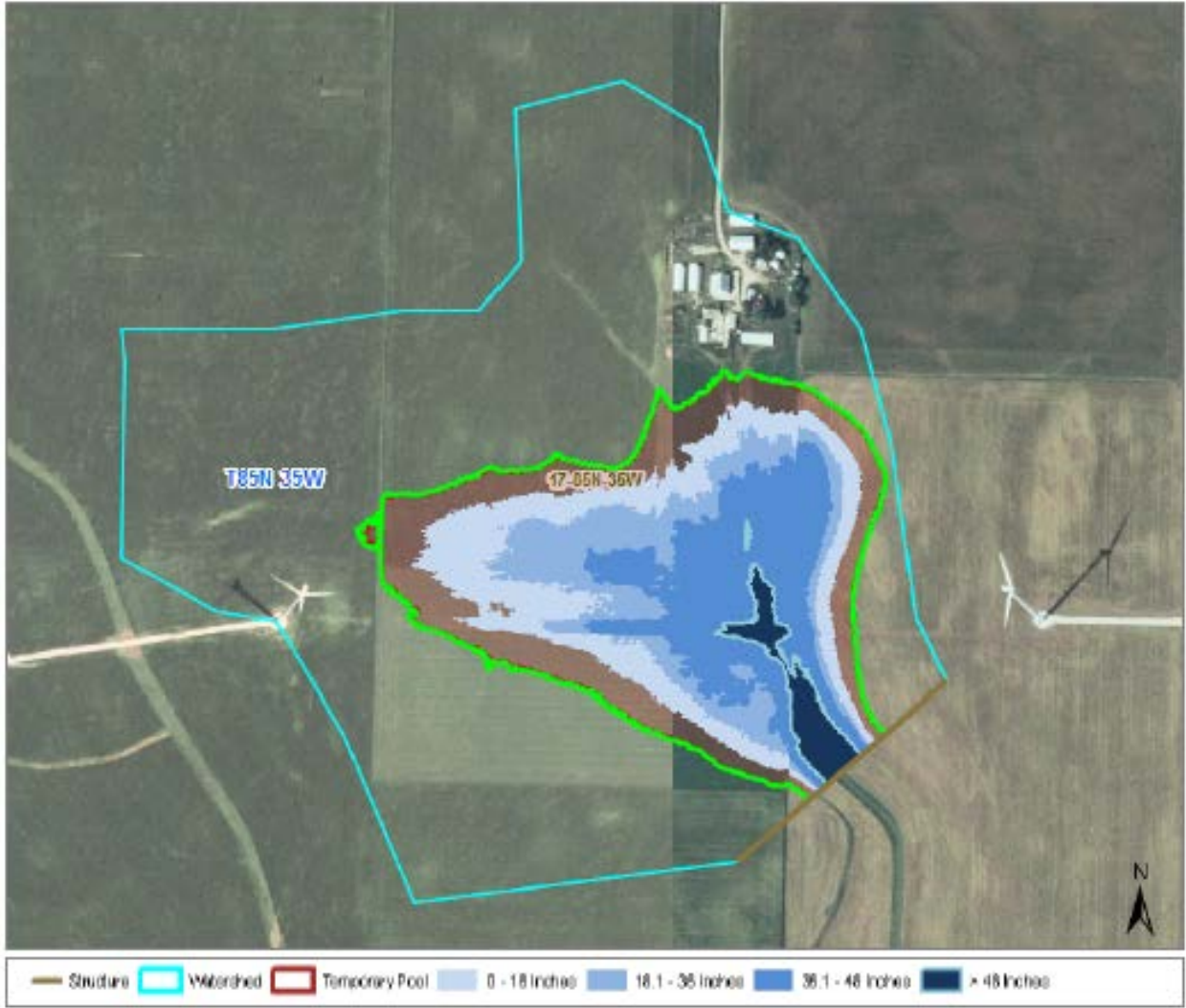
Map showing an example of a wetland area estimate generated from Agren's WetlandBuilder. Map provided by Agren.
