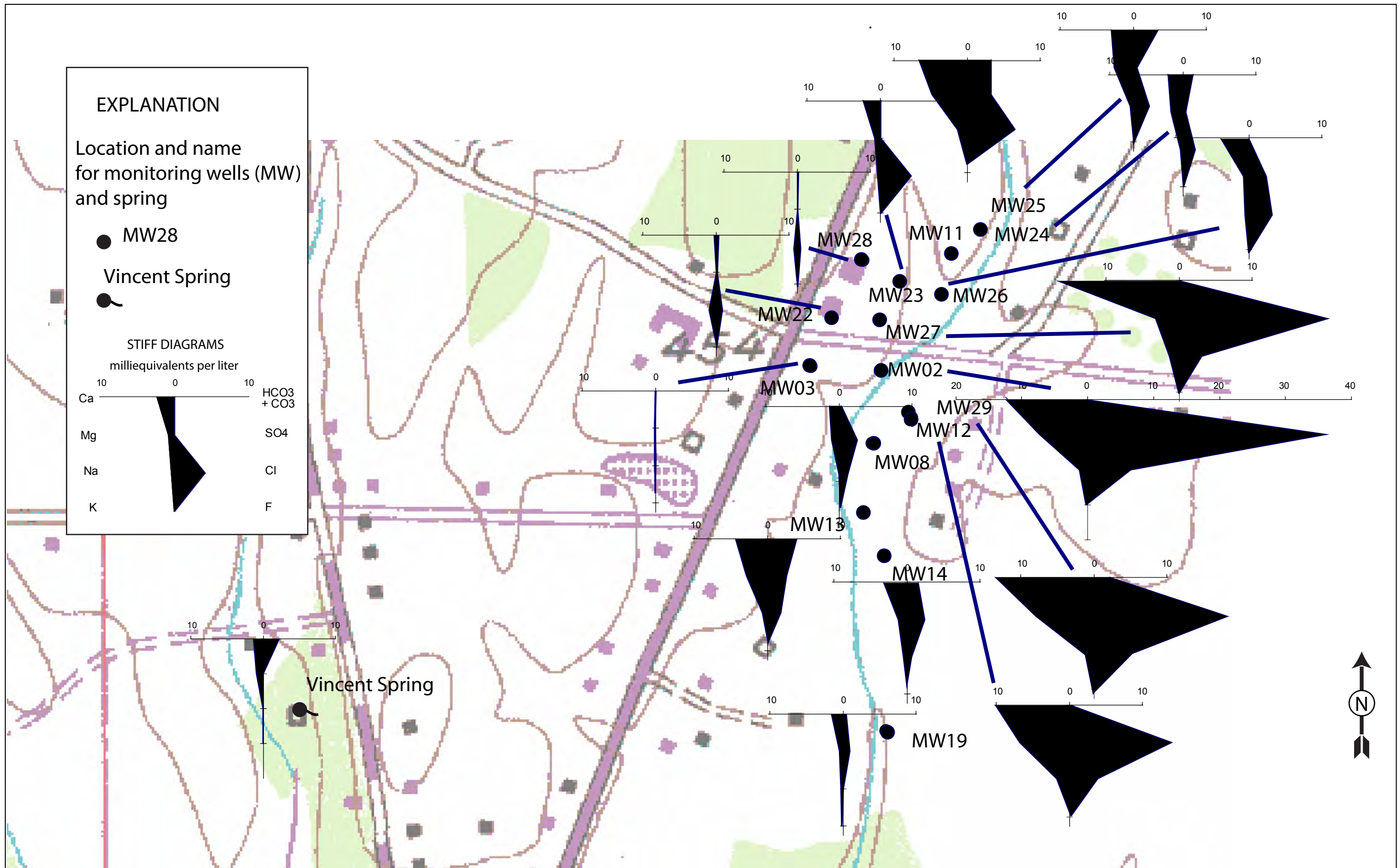
Plate 1. Stiff diagrams showing water type at Vincent Spring and monitor wells at the former Alabama Plating site, Vincent, Alabama, May 2007.
