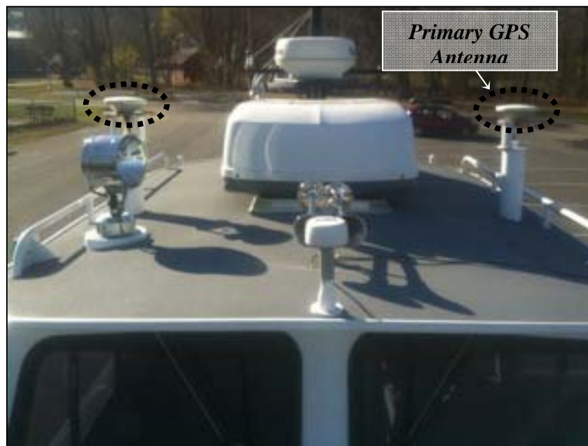
Figure 2: POS/MV Antenna Installation
