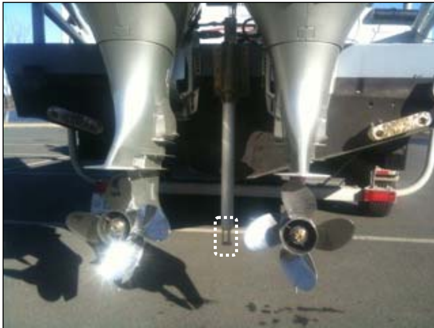
Figure 5: Surface Sound Speed Digibar Installation
