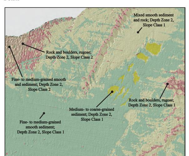
Figure 1. Detailed view of substrate classes mapped south of Soquel Point (see Box A, on map, for location): Depth Zone 2 (intertidal to 30 m), and Slope Classes 1 and 2 (0°–30°). Fine- to medium-grained smooth sediment is shown in shades of green; mixed smooth sediment and rock is shown in shades of tan; rock and boulder, rugose is shown in shades of pink and brown; and medium- to coarse-grained sediment is shown in shades of yellow.
