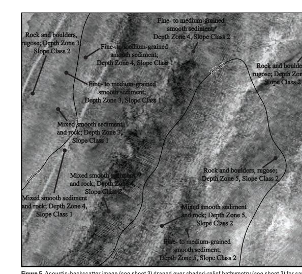
Figure 5. Acoustic-backscatter image (see sheet 3) draped over shaded-relief bathymetry (see sheet 2) for same area as figure 4 (Box B on map). Brighter areas indicate coarse-grained, rough, or hard seafloor; darker areas indicate unconsolidated (loosely packed) sediment. Parallel light-gray lines are data-processing artifacts. Interpreted substrate classes from figure 4 included for comparison. Bathymetric contours (100 m and 200 m) shown for depth reference.
