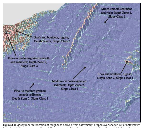
(see sheet 2) for same area as figure 1 (Box A on map). Rugosity values are displayed in muted "rainbow" color spectrum that ranges from purple (low rugosity) through green (medium rugosity) to red (high rugosity). Parallel lines of medium rugosity (green) are data-processing artifacts. Interpreted substrate classes from figure 1 included for comparison.
