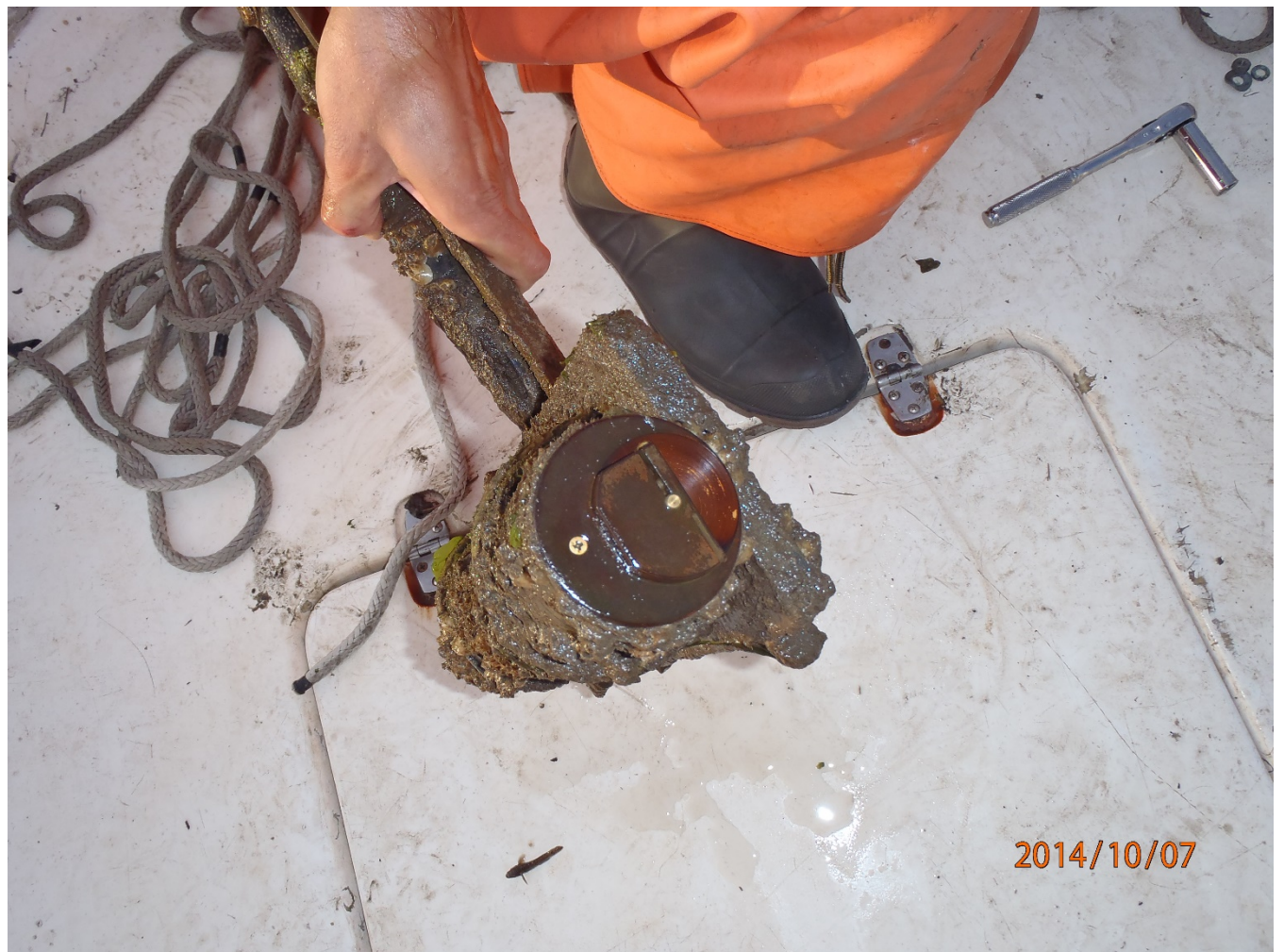
Figure 7. Sensor face of turbidity sensor upon recovery at Dinner Creek site on October 7, 2014, during turnaround of pole-mounted sensors. Anti-fouling wiper control kept optics area of the turbidity sensor relatively clean compared to rest of instrument body and mount.
