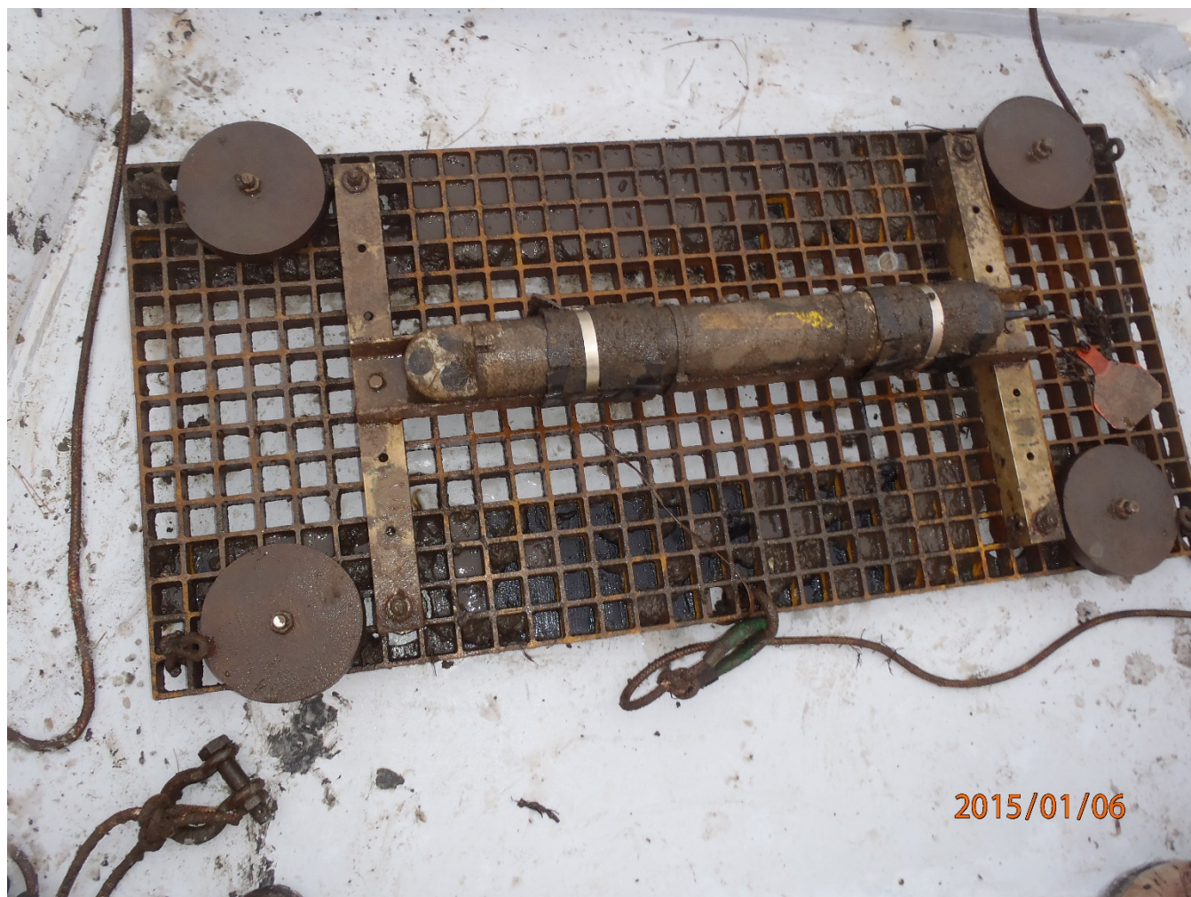
Figure 8. Recovered Aquadopp acoustic Doppler current profiler (ADCP) platform from Dinner Creek site on January 6, 2015. Light fouling, primarily from sediment, is present on instrument.
