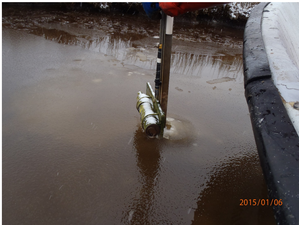
Figure 4. Pole-mounted sensors at Reedy Creek on January 6, 2015, just before recovery. Icing conditions are just beginning, and low-water event is exposing sensors to air. Water level got low enough to expose turbidity and temperature sensors on numerous occasions during the August 11, 2014, to January 6, 2015, deployment.
