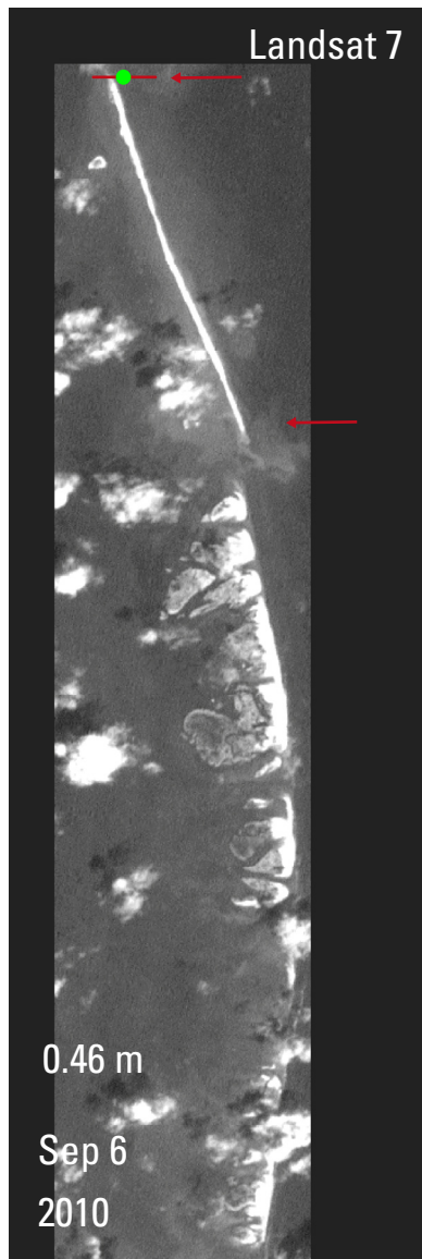
Figure 3. Landsat imagery of the berm on September 6, 2010, with a water level of 0.46 meter (NAVD 88). Green dot on red line indicates the location of the northern tip of the original constructed berm, and area between red arrows indicates length of berm used to calculate mean beach slope and berm toe.
