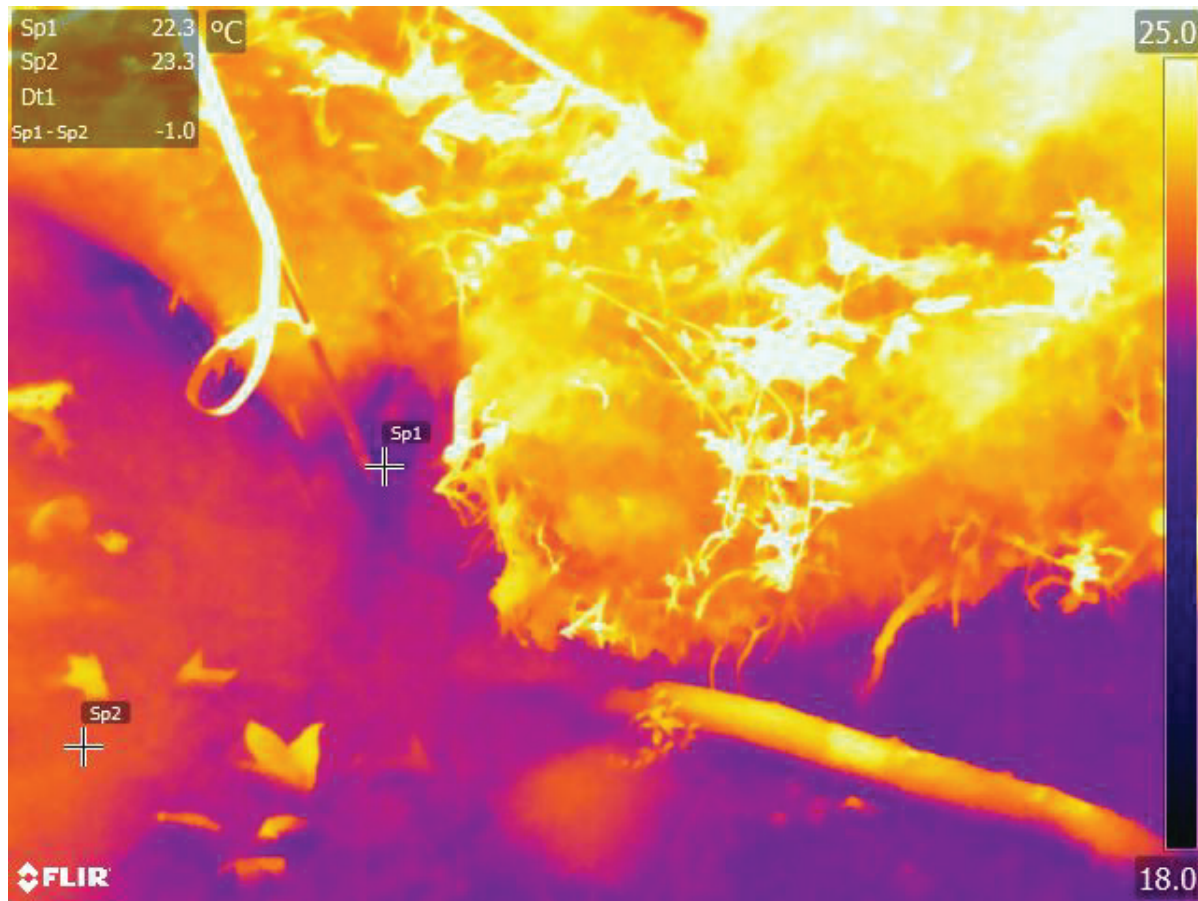
Figure 3-6. Infrared images captured by FLIR camera at site FS-06 to measure stream surface and bank seepage temperature differences in August/September 2014 near the Hemphill Road TCE National Priorities List Superfund site, Gastonia, Gaston County, North Carolina FS-01 to measure stream surface and bank seepage temperature differences in August/September 2014 near the Hemphill Road TCE National Priorities List Superfund site, Gastonia, Gaston County, North Carolina.
