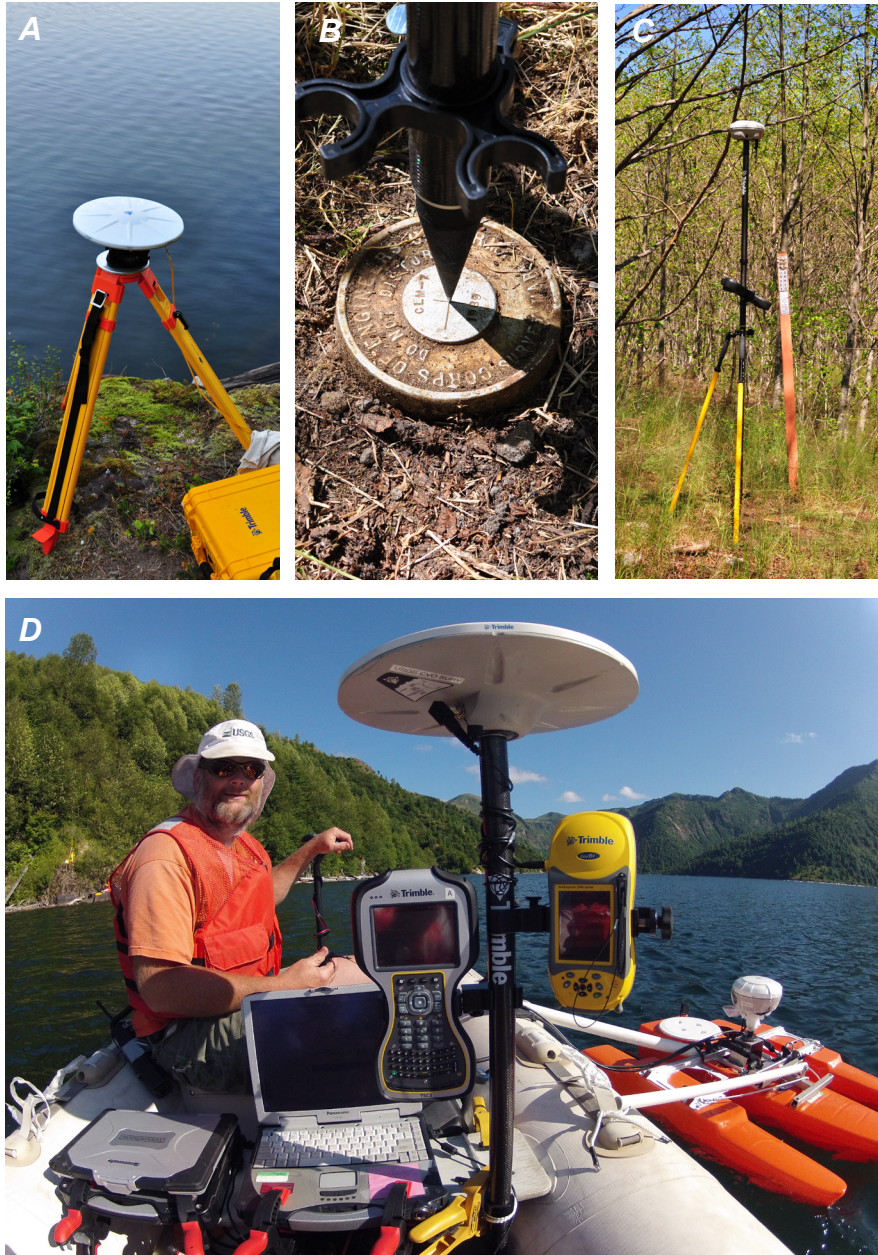
Figure 7. Photographs of field survey equipment. A , The primary global navigation satellite system (GNSS) base station. B , CLM-7 control monument. C , GNSS rover positioned over a control monument on the blockage. D , Wide-angle view from inside the survey boat showing mobile computers, GNSS equipment, and the acoustic Doppler current profiler (ADCP) positioned off the port side.
