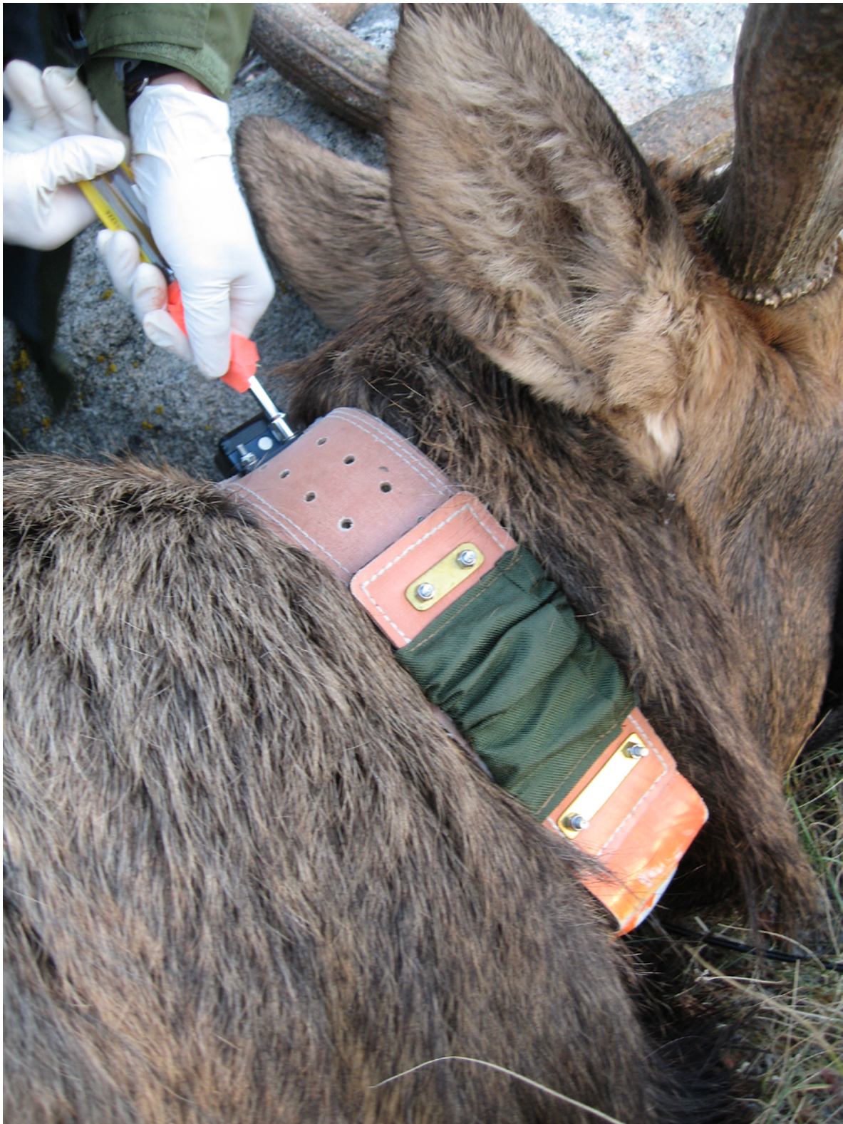
Figure 3. Modified bull elk radio collars showing expandable section developed by T. Johnson for elk population study in Rocky Mountain National Park, Colorado, 2008–2011. Photograph by K.A. Schoenecker, USGS.
