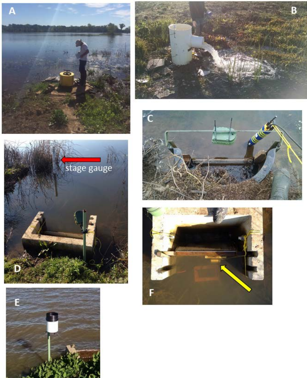
Figure 4. Photographs of the hydrology and water quality equipment used during the Cosumnes River Preserve mercury study. A, and B, source water inlets; C, check levee weir outfitted with water quality sonde; D, outlet water control structure and stage gauge (indicated by red arrow); E, rain gauge; F, fluorometer deployment (indicated by yellow arrow).
