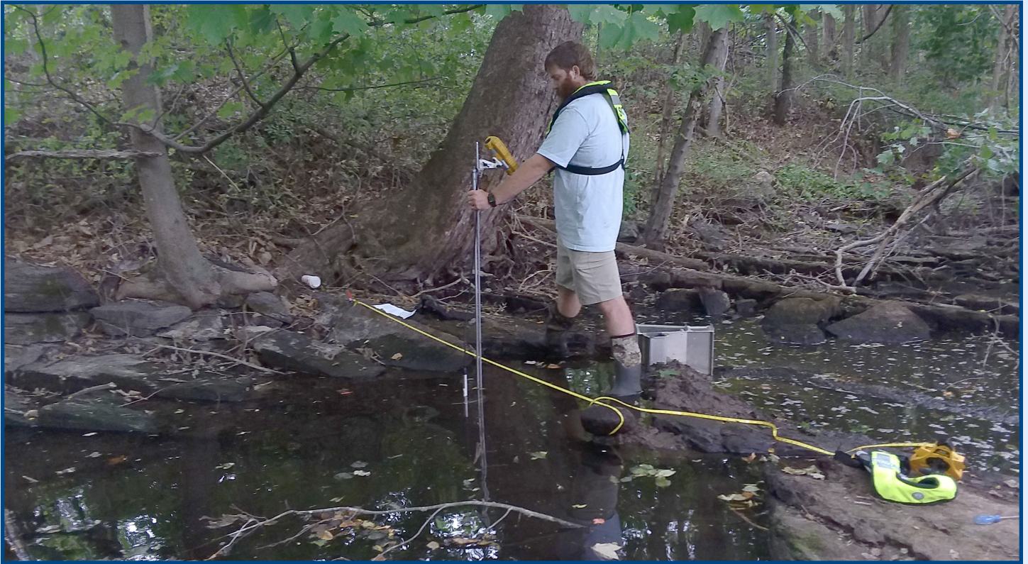
Photograph of streamflow measurement at Stony Brook near West Suffield, Connecticut, at U.S. Geological Survey streamgage 01184100 on September 18, 2020; photograph by Nigel Pepin, USGS.
