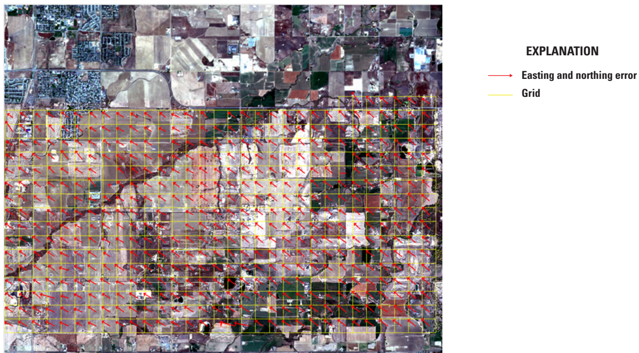
Figure 47. Relative geometric error comparison for Sentinel-2 and Pléiades Neo orthorectified image for the near-infrared band, Fort Lupton, Colorado.
