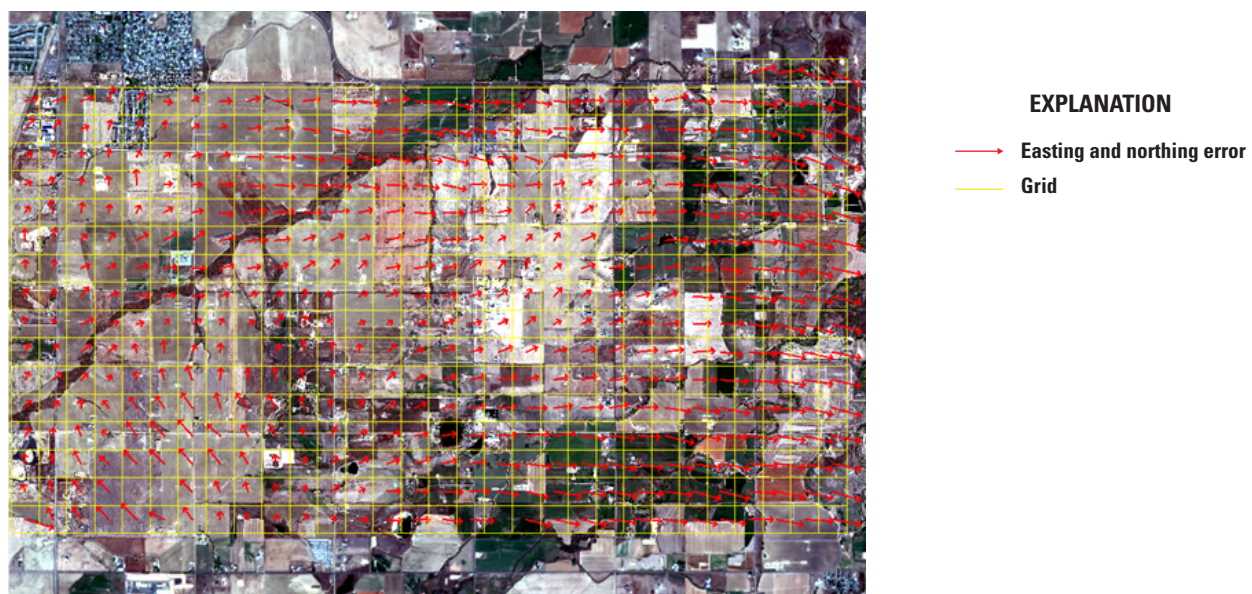
Figure 41. Relative geometric error comparison for Sentinel-2 and Pléiades Neo for the near-infrared band, Fort Lupton, Colorado.
