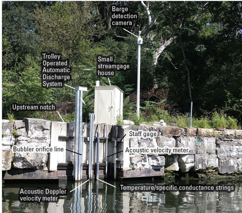
Gage house and instrumentation (Modified from Jackson (2018). Photograph by Clayton Bosch, U.S. Geological Survey.)
