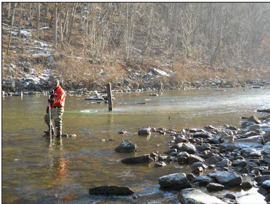
Figure 4. U.S. Geological Survey (USGS) hydrographers making concurrent streamflow measurements to compute springflow from the midchannel spring in Jackson River below Gathright Dam near Hot Springs, Virginia. Photograph by the USGS.
