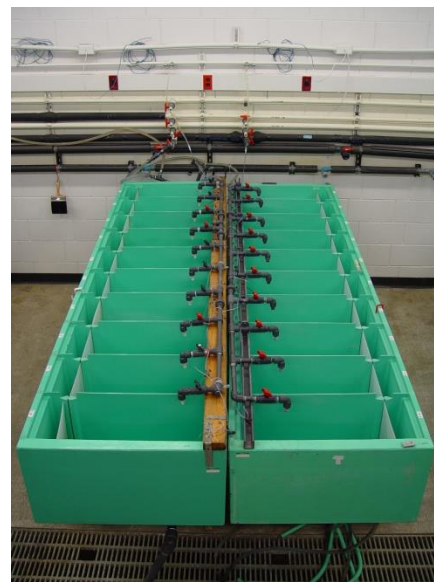
Figure 1. Experimental units (tanks) will be segregated into blocks of 10 test tanks contained within two ten-tank units. Individual tanks are separately plumbed and do not share water between tanks.
