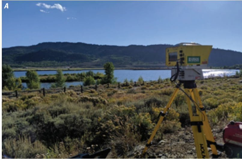
Figure 2. Illustration showing, A , photograph of terrestrial laser scanner used to collect data for the Windy Gap wildlife site in the western area of interest (AOI) site, B , the location of test sites chosen for field visits and detailed surveys using a combination of a terrestrial laser scanner, total station, and global navigation satellite system for data collection of mostly open, vegetated, and forested lands in the western AOI, and, C , the locations of mostly urban sites in the eastern AOI.
