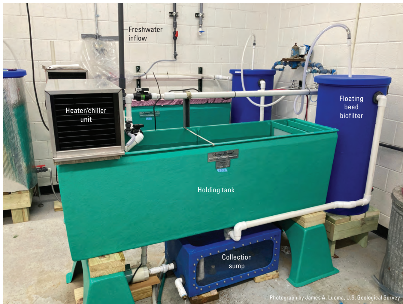
Figure 1. Recirculating system used to maintain Petromyzon marinus (sea lamprey) consisting of a holding tank, collection sump, floating bead biofilter, heater/chiller unit, and freshwater inflow.
