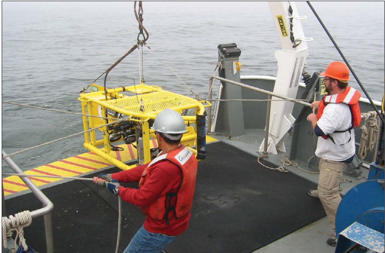
Figure 2. Photograph of camera sled being launched for ground-truth survey transect. Photograph by Guy R. Cochrane, 2009.
