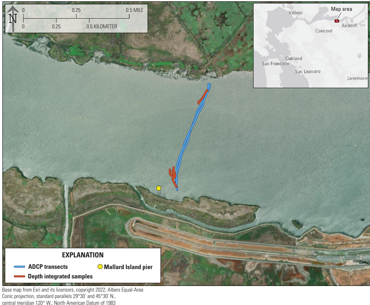
Figure 2. Map of the pier at the Mallard Island at Suisun Bay, California, streamgauge (U.S. Geological Survey Station 11185185, California Department of Water Resources Station MAL) and the February 2019 acoustic Doppler current profiler (ADCP) transects. Two ADCP transects (blue), and two depth-integrated vertical samples (red) were collected on the northern and southern extents (defined by thalweg) to investigate variability in suspended-sediment concentration distribution across the channel cross section. Depth-integrated samples consisted of one vertical sample collected using a D-96 sediment sampler.
