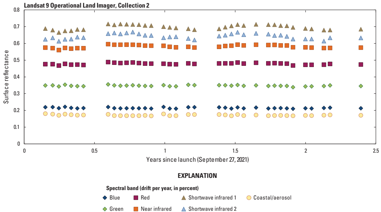
Figure 82. Graph showing Libya 4 pseudoinvariant calibration site surface reflectance trending, Landsat 9 Operational Land Imager, Collection 2.
