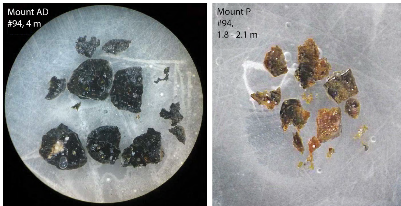
Figure 2. Photographs showing impact-melt particles in epoxy mounts used in this study. In the upper left of images is the sample identifier, drill hole number, and depth (in meters).
