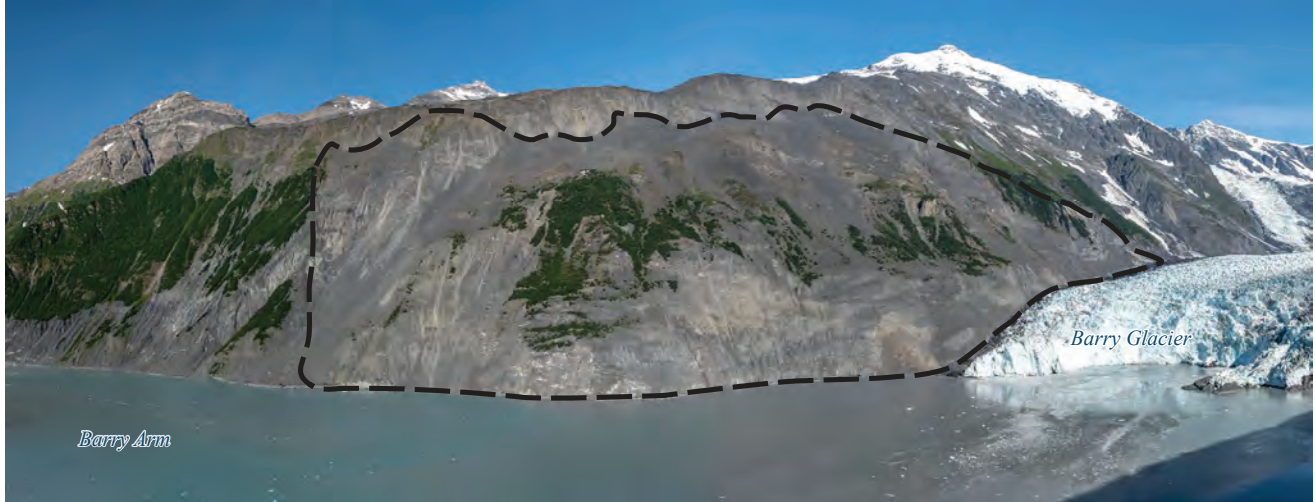
Figure 2. Panoramic photograph of the Barry Arm landslide, with the Barry Glacier terminus (north) to the right. The black dashed line indicates the approximate subaerial extent of the landslide complex. Photograph by Andrew Collins, U.S. Geological Survey.
