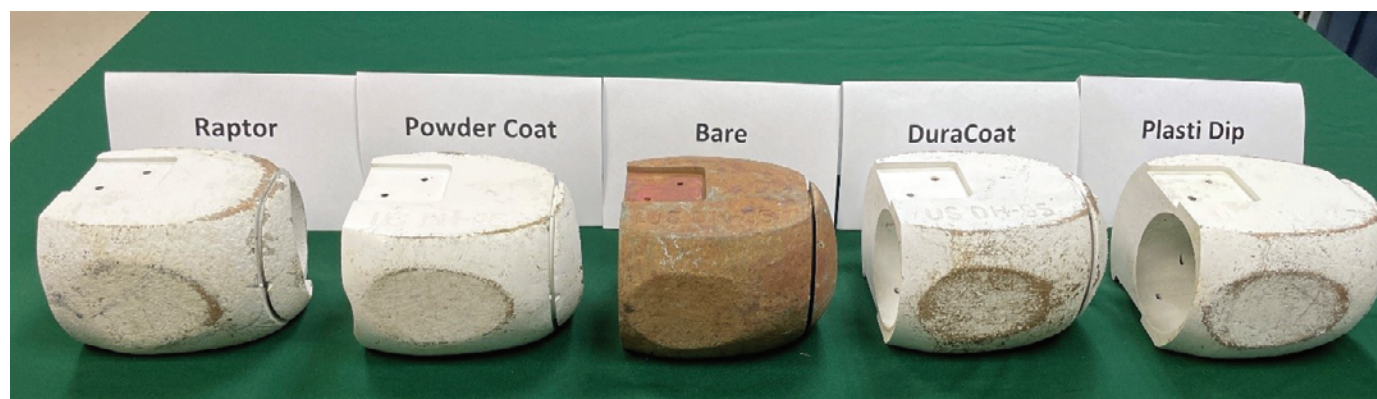
Figure 6. Photograph showing the damage to water-quality samplers after field use. Photograph taken by Alyssa Thornton, U.S. Geological Survey, on June 1, 2022.
