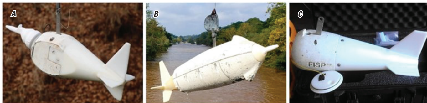
Figure 1. Photographs showing, A, DH-95, B, D-96, and, C, DH-2 water-quality samplers displaying moderate coating wear such as dents, abrasions, discoloration, and coating peeling. Photograph A taken by Ken Hyer, U.S. Geological Survey (USGS), on December 10, 2007. Photograph B taken by Jimmy Webber, USGS, on September 20, 2018. Photograph C taken by Jimmy Webber, USGS, on June 05, 2013.
