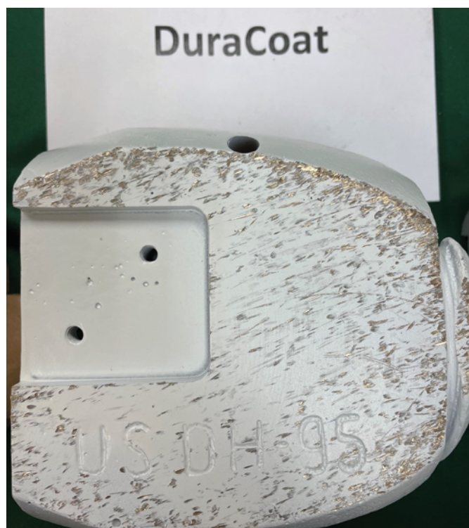
Figure 3. Photograph showing damage to the side of the DuraCoat sampler (fins removed) following the controlled wear test. Photograph taken by Alyssa Thornton, U.S. Geological Survey, on December 2, 2020.
