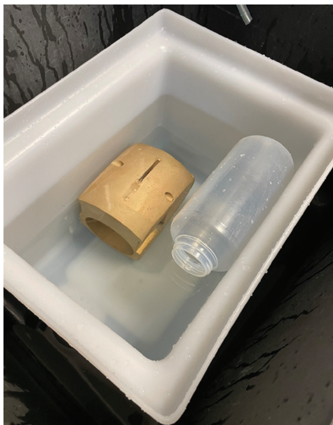
Figure 2. Photograph showing blank water-quality sample processing from a wash basin using a bare sampler. Photograph taken by Alyssa Thornton, U.S. Geological Survey, on December 2, 2020.
