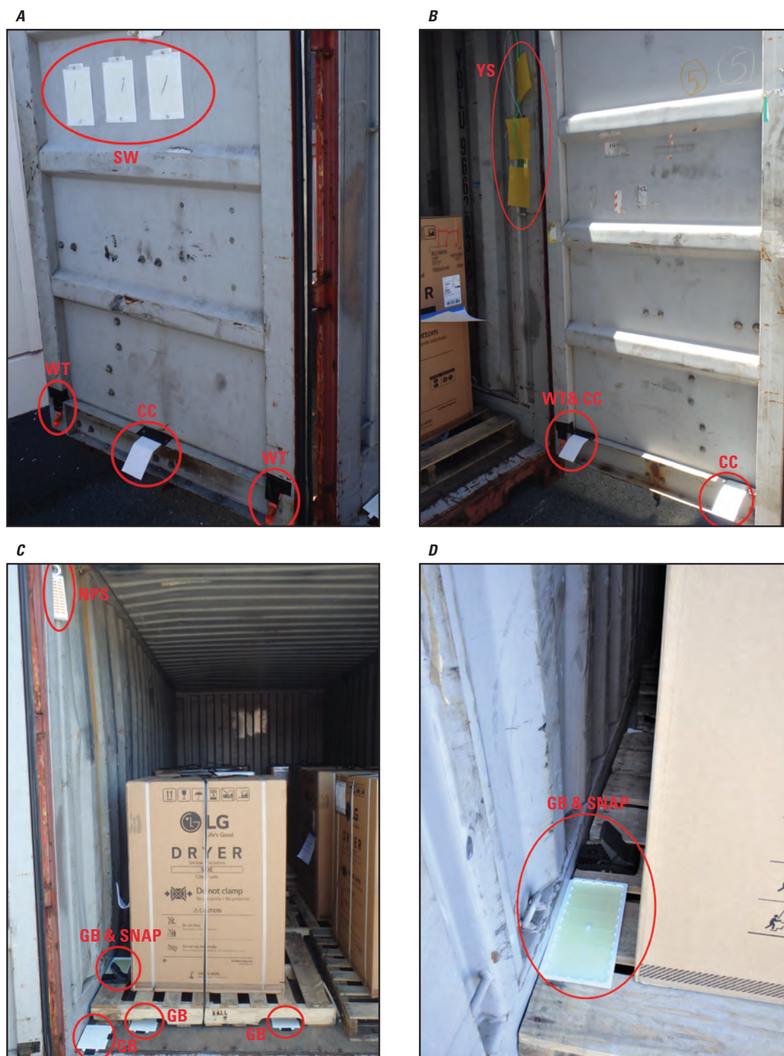
Figure 7. A suite of biosecurity tools that was placed in each 2018 Wake Atoll resupply container at Joint Base Pearl Harbor–Hickam during the stuffing phase as they were stuffed with cargo including A , two wax tags (WT), one chew card (CC) and three glue board traps were placed on one container door (SW); B , one WT, two CC, and three yellow glue board traps (YS) were placed on another container door; C , three glue board traps (GB) were taped to the container floor, one pest strip (NPS) was attached to the upper left lashing bar, one snap trap (SNAP), and one GB were placed on a pallet; and D , close-up of a SNAP and GB on pallet. The SNAP, NPS, and one GB are tools required by the Wake Island Biosecurity Management Plan, and the WT, CC, YS, SW, and three additional GB were added as part of the evaluation of the efficacy of this plan. Photographs by S.A. Hathaway, U.S. Geological Survey.
