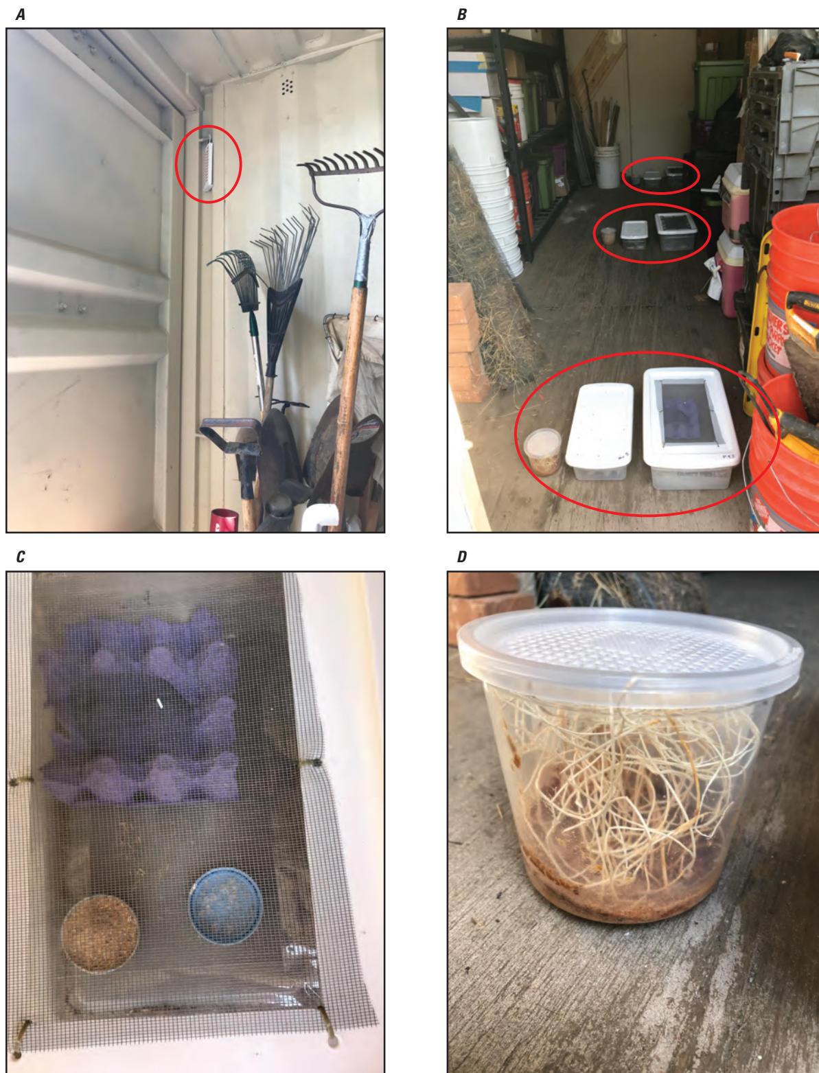
Figure 13. Components of a shipping container trial for evaluating the efficacy of using dichlorvos impregnated pest strips as a biosecurity tool, including A , location of pest strip (circled in red) hanging inside treatment shipping container at a front top tiedown provision; B , view from door of treatment shipping container showing insect enclosures (circled in red) placed at three distances from where pest strips were placed; C , cockroach and cricket enclosures containing a dish of commercial roach and cricket chow as well as a dish of insect water gel crystals; and D , fruit fly containers containing commercial culture media. Photographs by S.A. Hathaway, U.S. Geological Survey.
