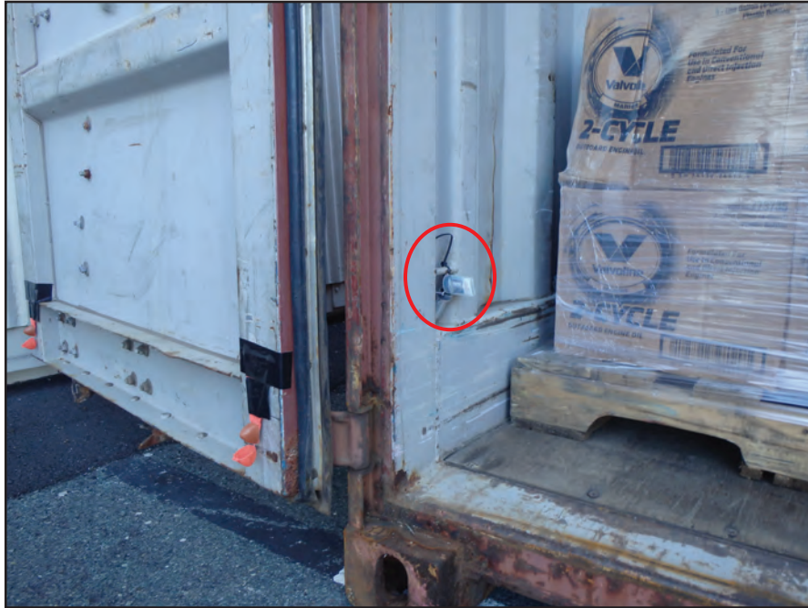
Figure 8. Temperature loggers (circled in red) placed in a stuffed shipping container used for the 2018 Wake Atoll resupply shipment. Photograph by S.A. Hathaway, U.S. Geological Survey.
