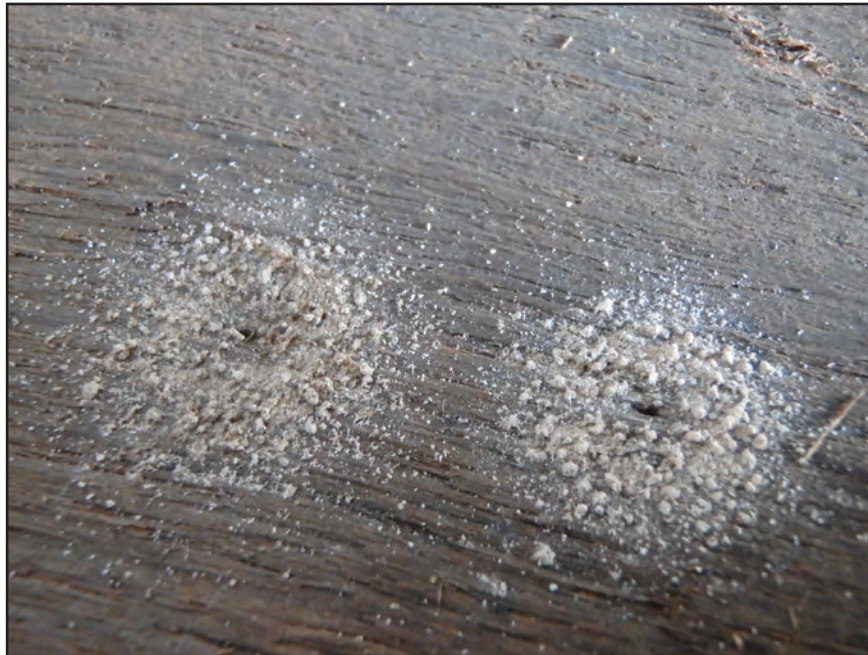
Figure 16. Example of boreholes detected in the floorboards in empty shipping containers during inspections before stuffing with cargo for Wake Atoll resupply, spring 2018. Photograph by S.A. Hathaway, U.S. Geological Survey.
