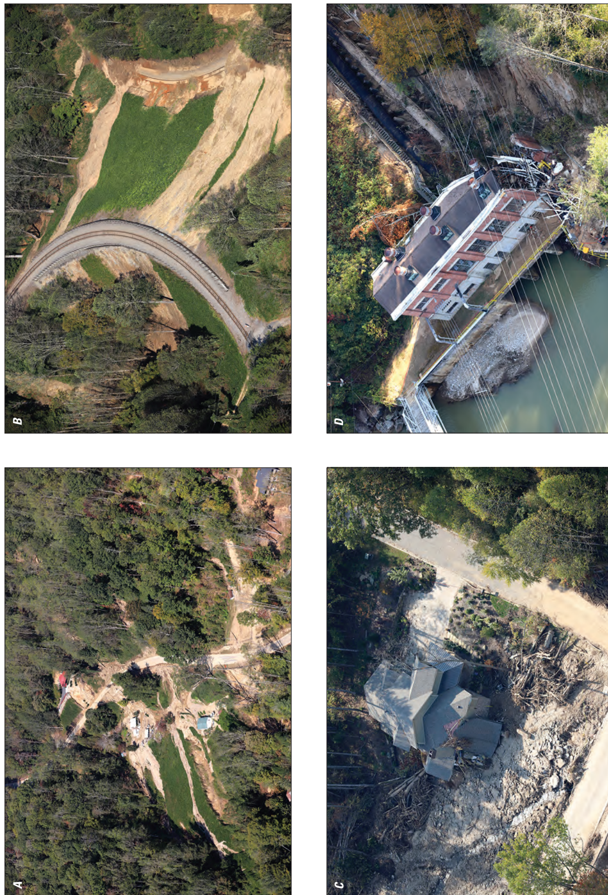
Figure 2. Photographs showing examples of homes and infrastructure affected by landslides and mudflows observed during reconnaissance flights in North Carolina. A. High concentration of impactful landslides in Bat Cave, 35.463°, -82.285°. B. Failures of engineered slope along railroad (left) inundating a lower-elevation section of track (right), 35.656°, -82.242°. C. House damaged by mudflow near Black Mountain, the road has been cleared of debris, 35.593°, -82.316°. D. Hydropower structure damaged by a landslide, 35.248°, -82.391°. Coordinates indicate the approximate location of the photographer (Photographs by S. Slaughter, U.S. Geological Survey).
