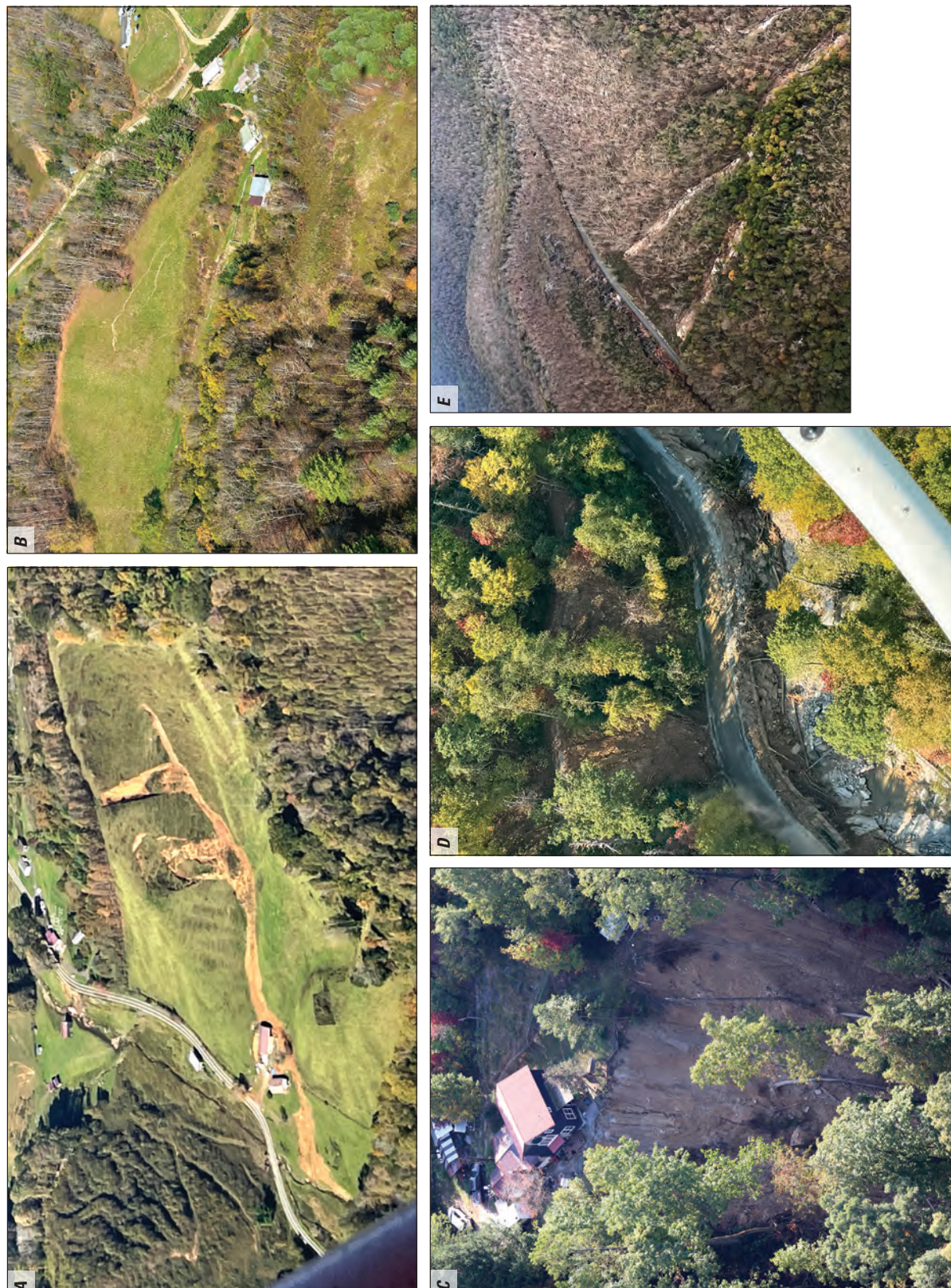
Figure 5. Photographs showing examples of ongoing landslide hazards in North Carolina. A, Destabilized material remaining in the landslide source area, 36.512°, -81.568° (Photograph by F. Rengers, U.S. Geological Survey); B, cracks indicating a landslide started to form, 36.290°, -81.777° (Photograph by J. Godt, U.S. Geological Survey); C, undercut slope resulting in destabilization of the structure and areas above, 35.542°, -82.204° (Photograph by S. Slaughter, U.S. Geological Survey); D, a road that was undercut and destabilized by flood erosion and prone to continued material failing from the slope above, 35.466°, -82.305° (Photograph by K. Allstadt, U.S. Geological Survey); E, Trees blowdown that may increase susceptibility to future debris flows due to loss of root strength, two mudflow source areas are visible to the left, 35.688°, -82.404° (Photograph by F. Rengers, U.S. Geological Survey). Coordinates indicate the approximate location of the photographer.
