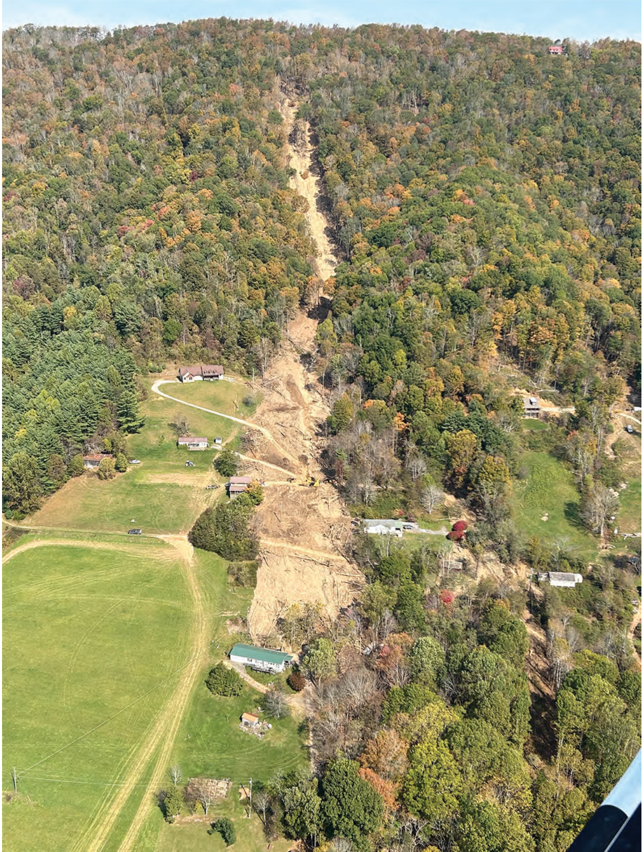
Figure 3. Photograph showing a landslide that transitioned into a mudflow that damaged structures near Boone, North Carolina. Approximate coordinates of the photographer were 36.259°, -81.744° (Photograph by J. Godt, U.S. Geological Survey).
