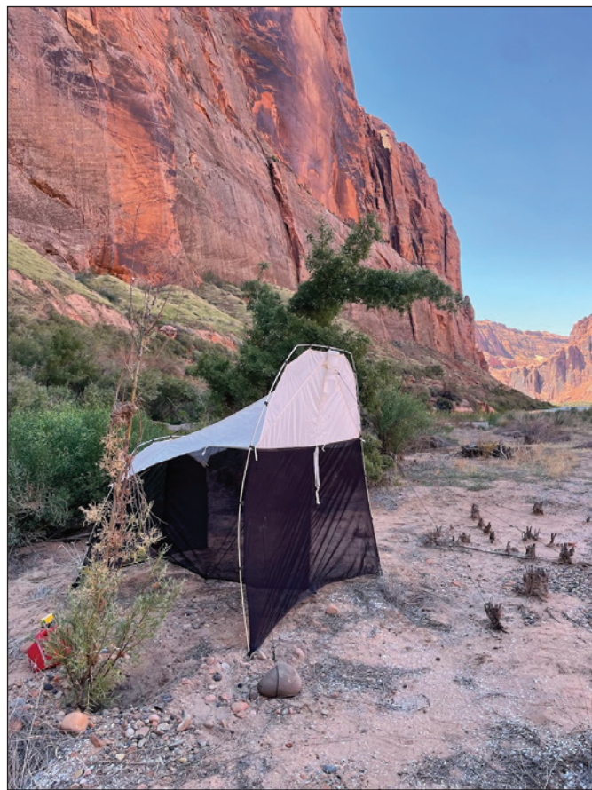
Figure 3. Photograph of a malaise trap deployment at the Upper Slough. These traps are 1.7 meters in length, 1.2 meters tall, and have a medial dividing mesh wall that directs flying insects upwards into a mesh apex that exits to a plastic sampling container filled with ethanol. Photograph by Anya Metcalfe, U.S. Geological Survey.
