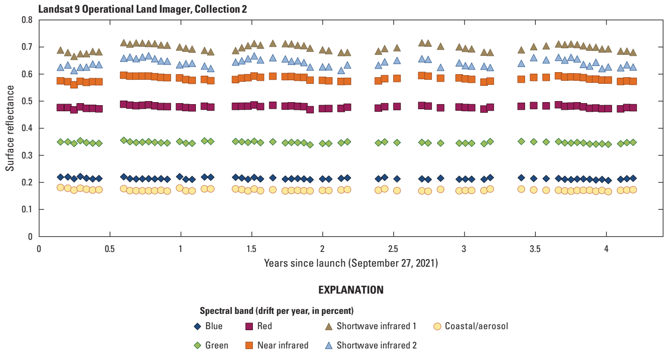
Figure 82. Graph showing Libya 4 pseudoinvariant calibration site surface reflectance trending, Landsat 9 Operational Land Imager, Collection 2.
