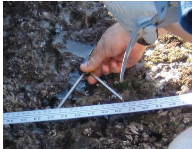
Figure 3. Black abalone ( Haliotis cracherodii ) shell length is measured to the nearest millimeter by using divider calipers and a ruler, San Nicolas Island, California. Photographs taken by M.C. Kenner, U.S. Geological Survey, January 22, 2019.
