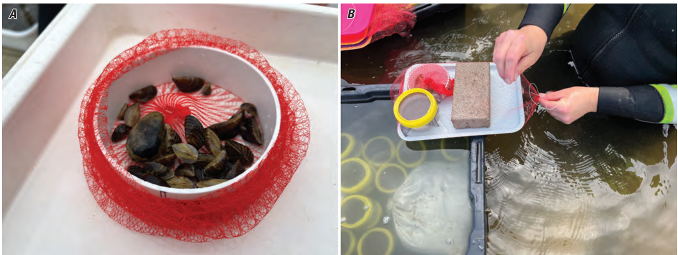
Figure 4. Photographs showing (A) sentinel Dreissena polymorpha (zebra mussels) caged within a mesh bag that was held open by a rigid plastic ring and (B) zebra mussel cages placed onto a tray along with a brick. The tray and contents were placed into a second mesh bag for containment. Within each plot, 12 trays were deployed.
