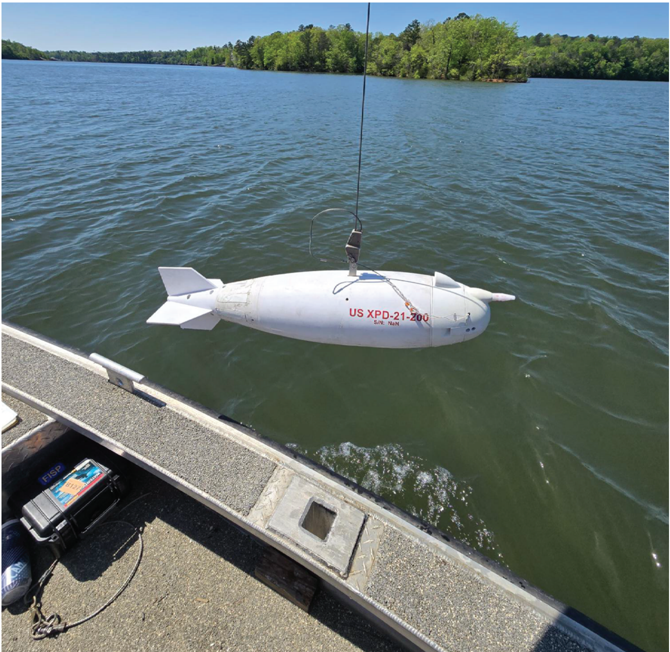
Figure 4. Photograph of the US XPD-24-200 sampler hanging from the crane on Lake Tuscaloosa, Alabama. Photograph by U.S. Geological Survey.
