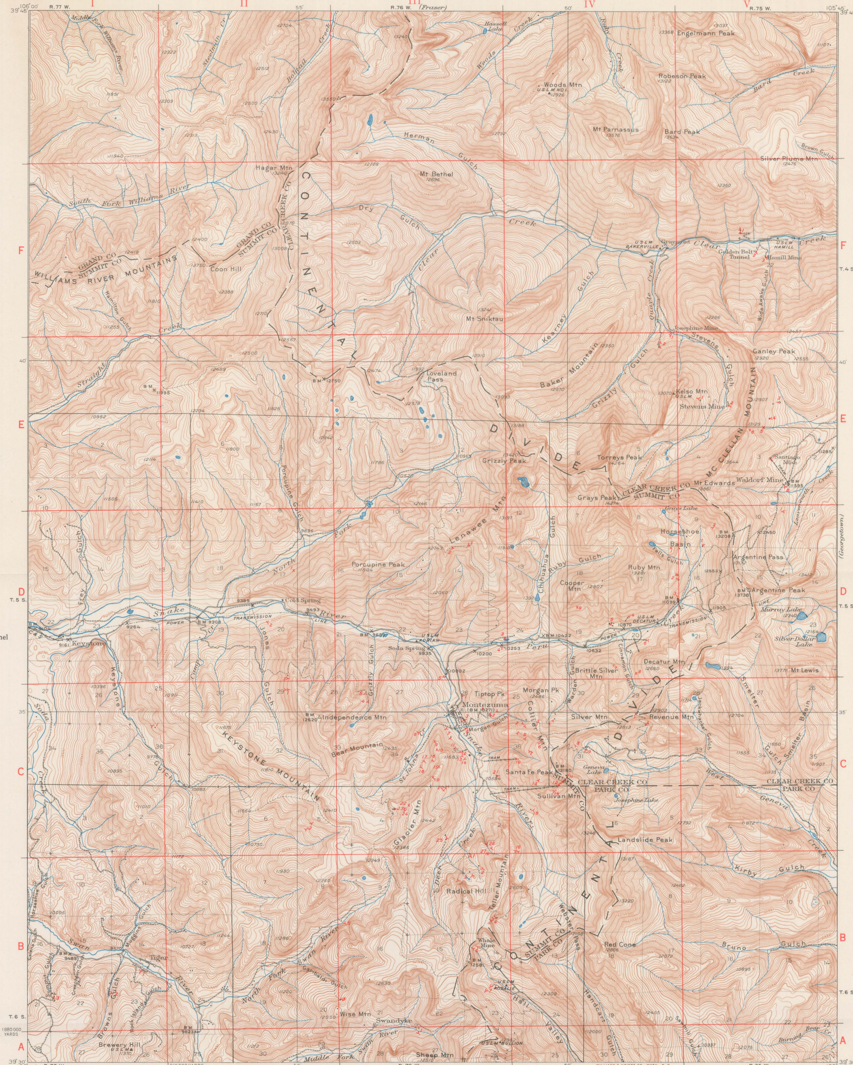
Topography by Albert Pike, H.H. Hodgeson, Max J. Gleisner, and from Breckenridge special map Surveyed in 1924 TOPOGRAPHIC MAP OF MONTEZUMA QUADRANGLE, COLORADO, SHOWING MINE LOCATIONS Scale 62500 Contour interval 50 feet Datum is mean sea level 1935 Polyconic projection, North American datum 5000 yard grid based upon U.S. zone system. E
