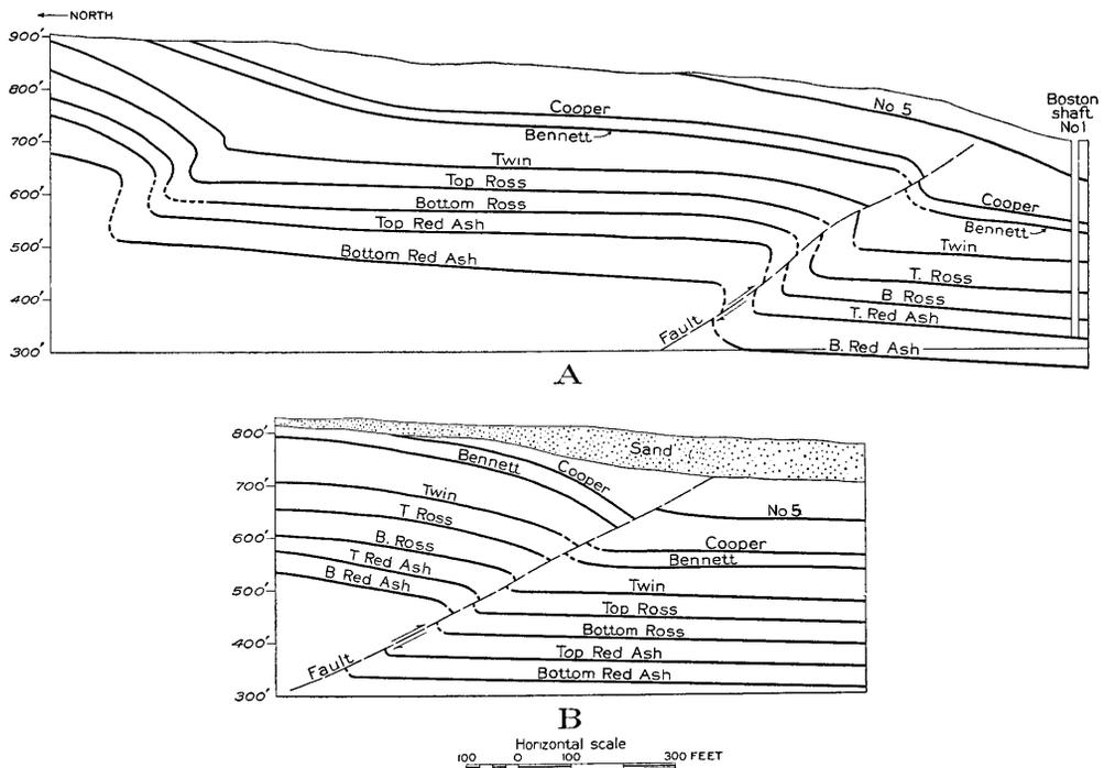
FIGURE 17.—Sections showing fault in Loree colliery, Plymouth: A, North of Boston shaft; B, West of Boston shaft.
