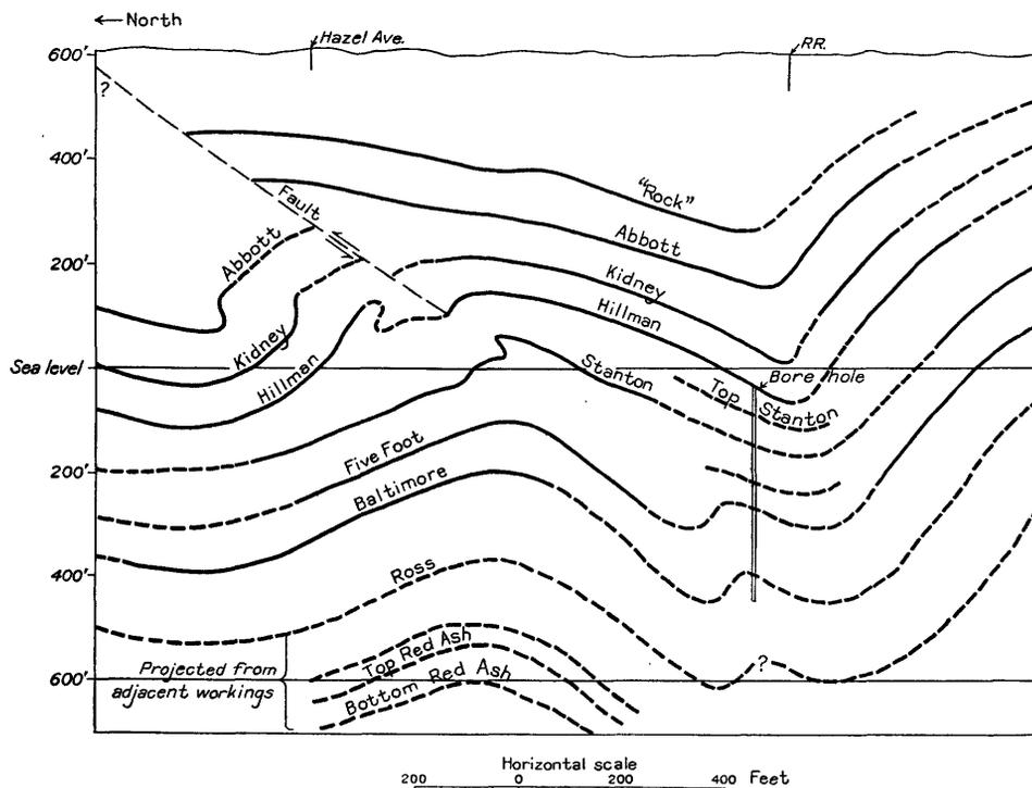
FIGURE 14.—Section in the southwestern part of South Wilkes-Barre colliery. Compiled from section by Glen Alden Coal Co. Broken lines are hypothetical; solid lines represent mined coal.
