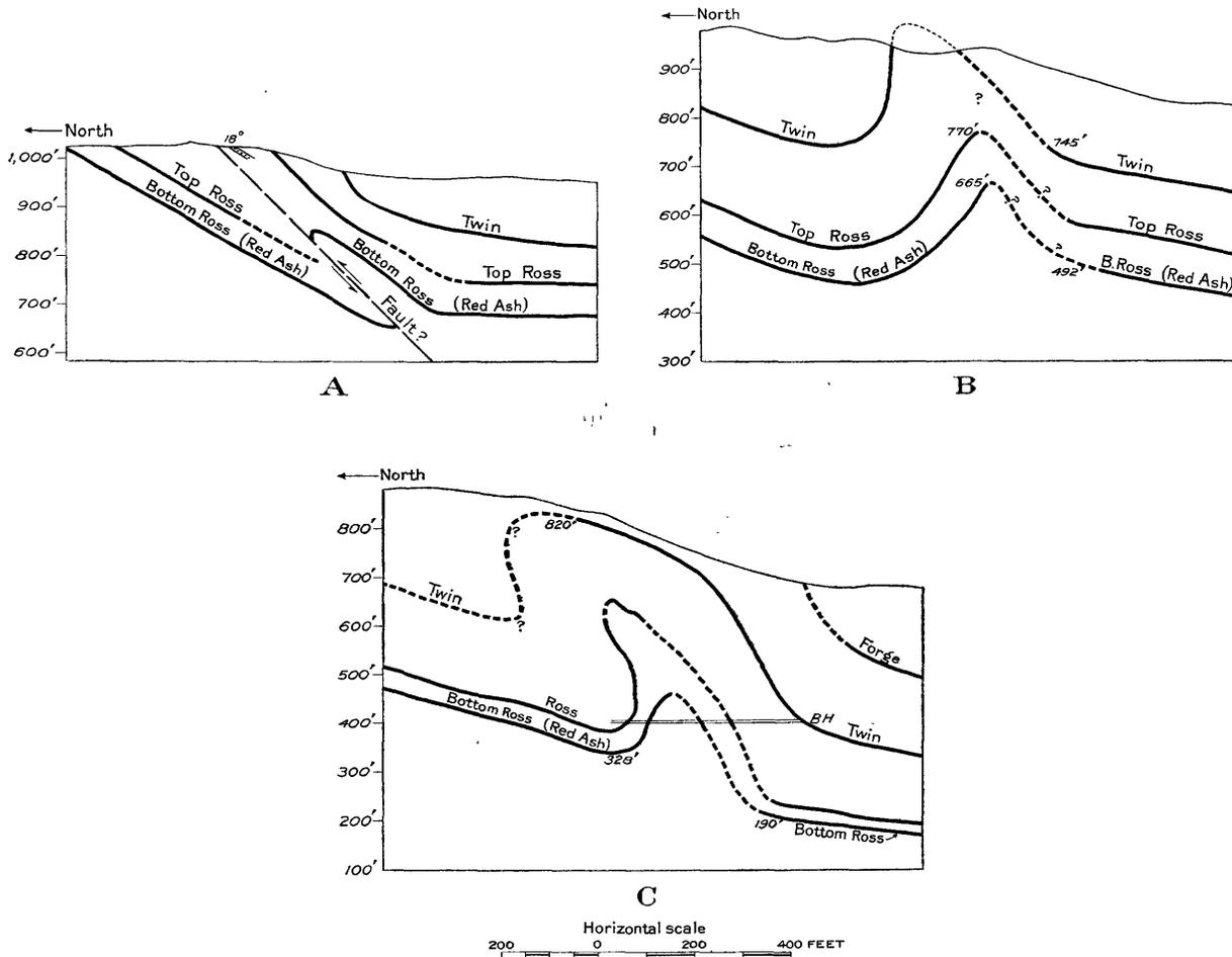
FIGURE 10.—Sections across anticline north and west of Glenlyon: A, Along west boundary of Glenlyon colliery; B, just north of shaft 7; C, north of shaft 6. Compiled from sections by Susquehanna Coal Co. BH, Borehole. Broken lines are hypothetical; solid lines represent mined coal. Altitudes of coal beds given are at end workings.
