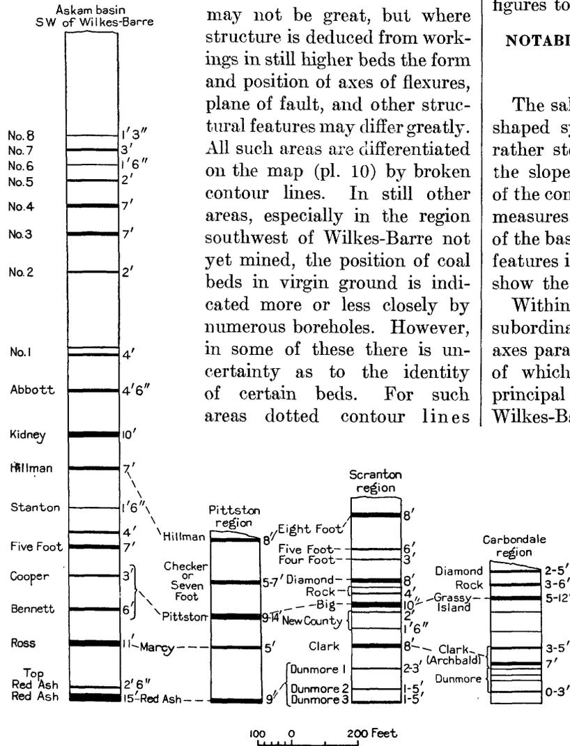
FIGURE 7.—Principal coal beds in different parts of the Northern Anthracite coal basin. In some places the thicknesses as given include waste.
