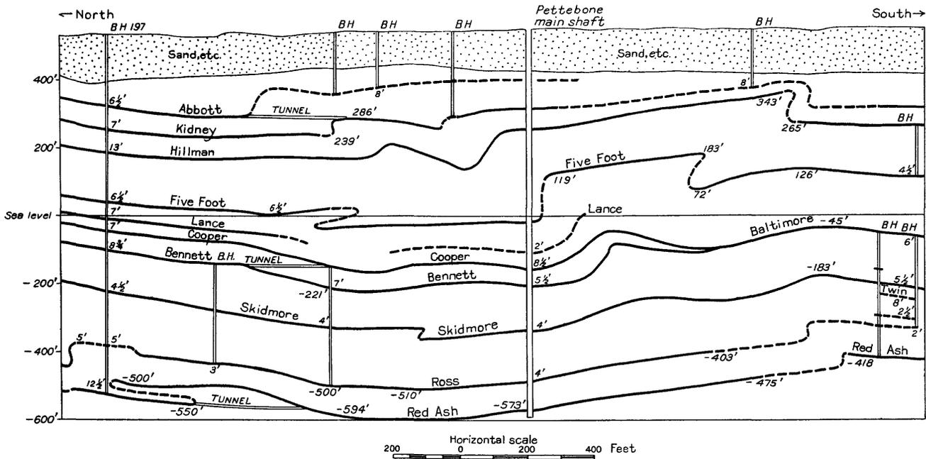
FIGURE 18.—Section of Pettebone colliery, Kingston. BH, Borehole. Broken lines are hypothetical; solid lines represent mined coal. Altitudes and thicknesses of coal beds are given.
