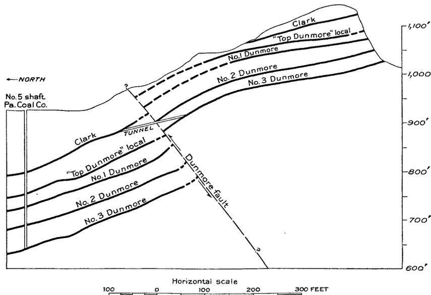
FIGURE 19.—Section across Dunmore fault just south of Pennsylvania Coal Co. shaft 5.
