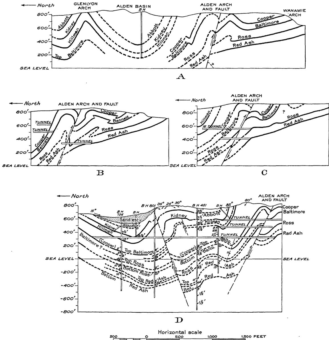
FIGURE 9.—Sections across Alden arch and fault in Wanamie colliery north of shaft 19: A, 1,300 feet east of section D (shows also some relations of Alden basin and Glenlyon arch); B, about 400 feet east of section D, near tunnel 16; C, 800 feet east of section D; D, N. 10° W. of Wanamie shaft 19. BH, Borehole. Broken lines are hypothetical; solid lines represent mined coal. Thicknesses of coal beds given are in boreholes and include waste.
