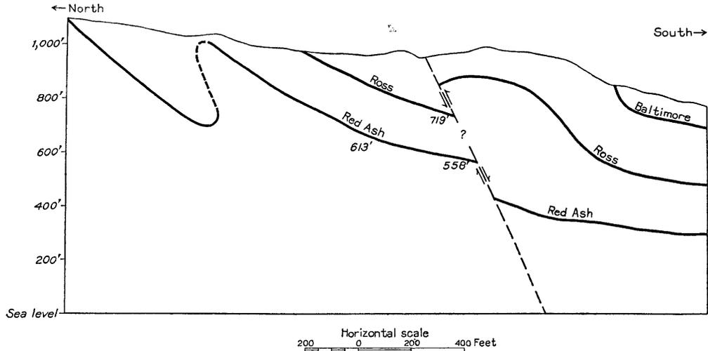
FIGURE 16.—Section across fault and roll in the northwestern part of Nottingham colliery, Plymouth. Figures given are altitudes of coal beds.
