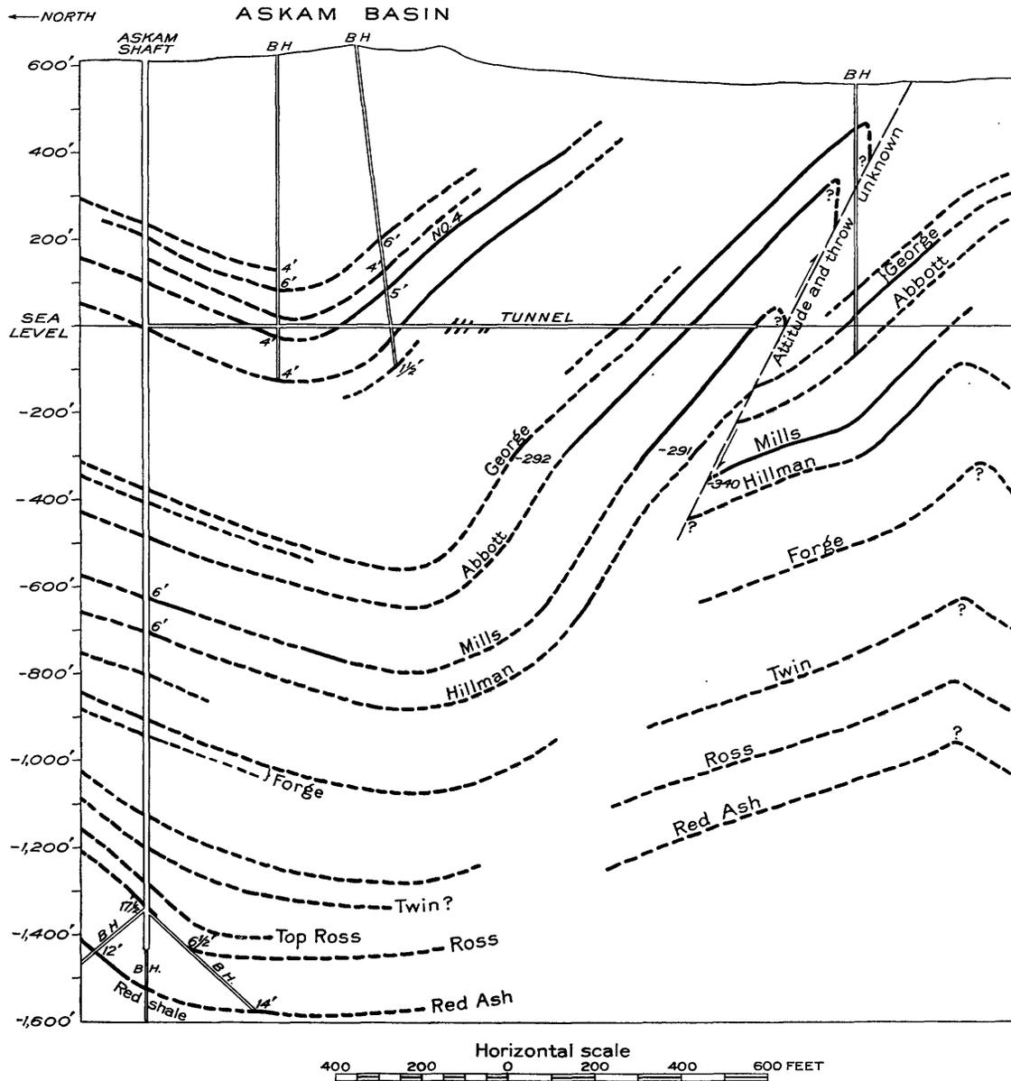
FIGURE 12.—Section from Askam shaft southward, showing probable relations of the Alden north fault and the Alden arch. From section by the Glen Alden Coal Co., slightly modified. BH, Borehole. Broken lines are hypothetical; solid lines represent mined coal. Altitudes given are at end workings; thicknesses of coal beds as given in boreholes include waste.
