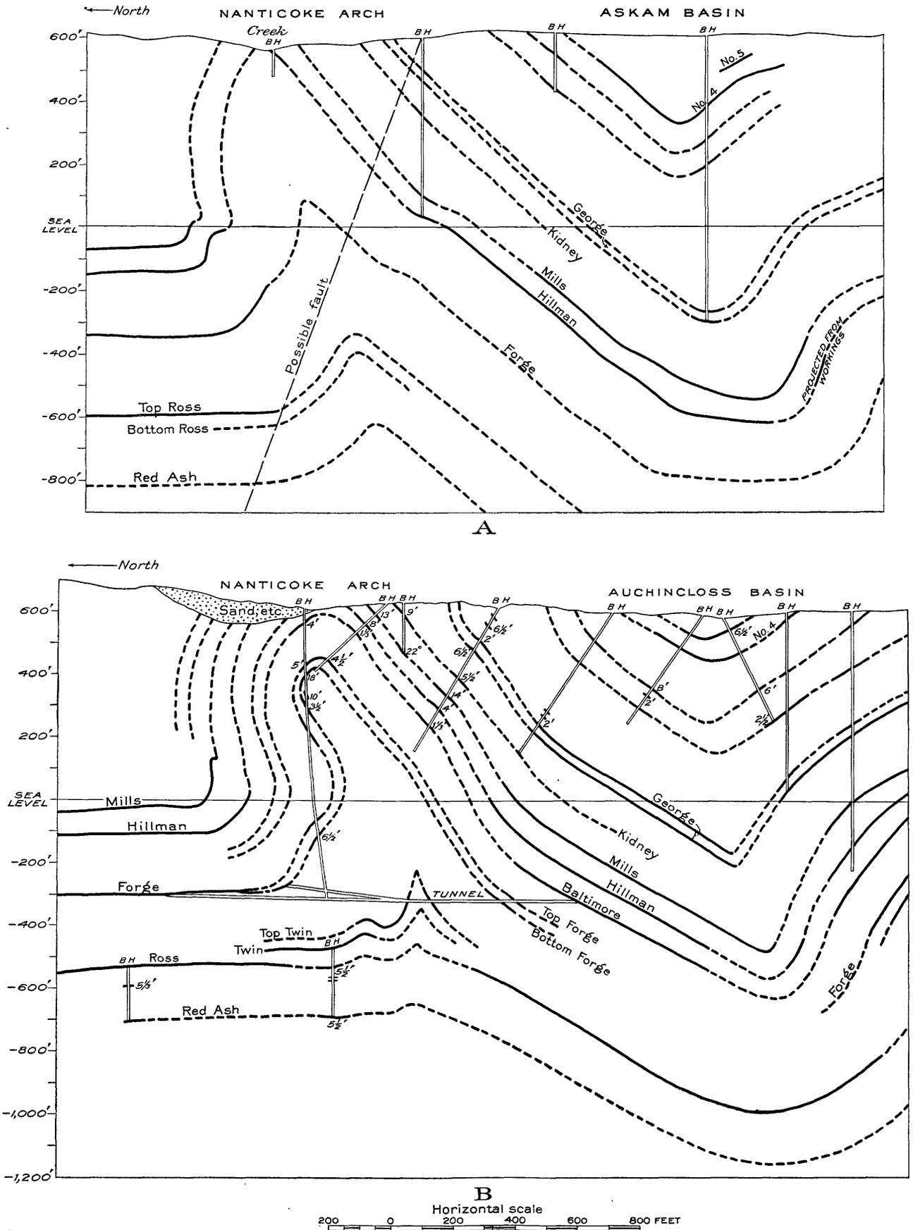
FIGURE 11.—Sections across the eastern extension of the Nanticoke arch and the Auchincloss-Askam basin: A, North of Truesdale shaft; B, 2,500 feet east of Auchincloss shaft. Compiled from sections by Glen Alden Coal Co. BH, Borehole. Broken lines are hypothetical; solid lines represent mined coal. Thicknesses of coal beds as given in boreholes include waste.
