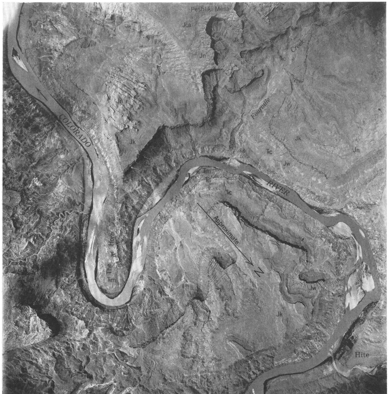
FIGURE 87.—Vertical view of the Colorado River below Hite. At the mouth of each tributary is a sand bar. Tm, Moenkopi formation; Ts, Shinarump conglomerate; Tc, Chinle formation; Jw, Wingate sandstone; Jk, Kayenta formation; Jn, Navajo sandstone; Jca, Carmel formation. Peshliki Mesa is about 2,000 ft higher than the river. Horizontal scale, about 2 in. equals 1 mile. Photograph by Fairchild Aerial Surveys.
