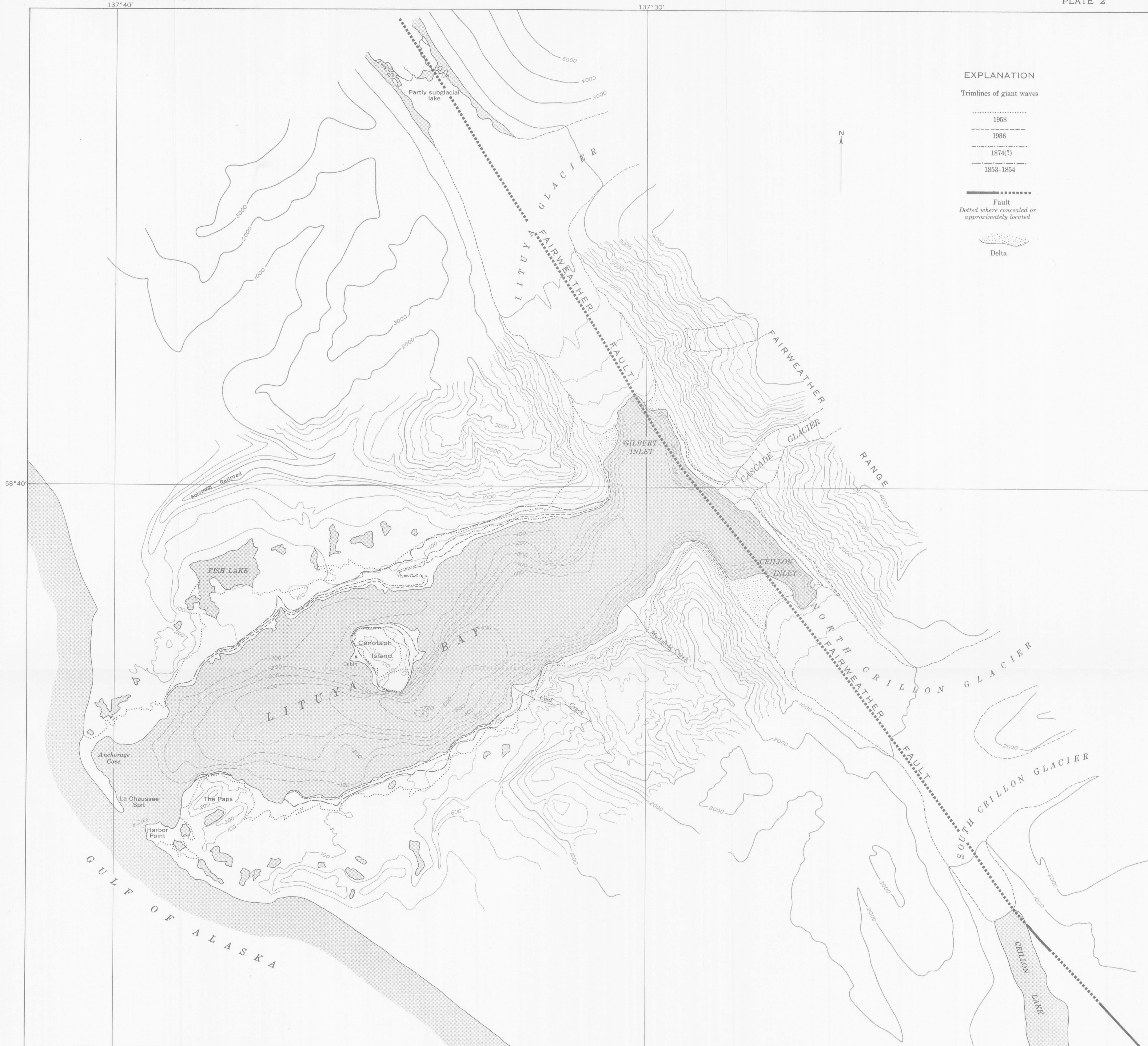
MAP OF LITUYA BAY AND ADJOINING AREA, SHOWING SUBAERIAL AND SUBMARINE TOPOGRAPHY, TRACE OF FAIRWEATHER FAULT AND TRIMLINES OF KNOWN GIANT WAVES AS MAPPED IN THE FIELD AND FROM PHOTOGRAPHS
