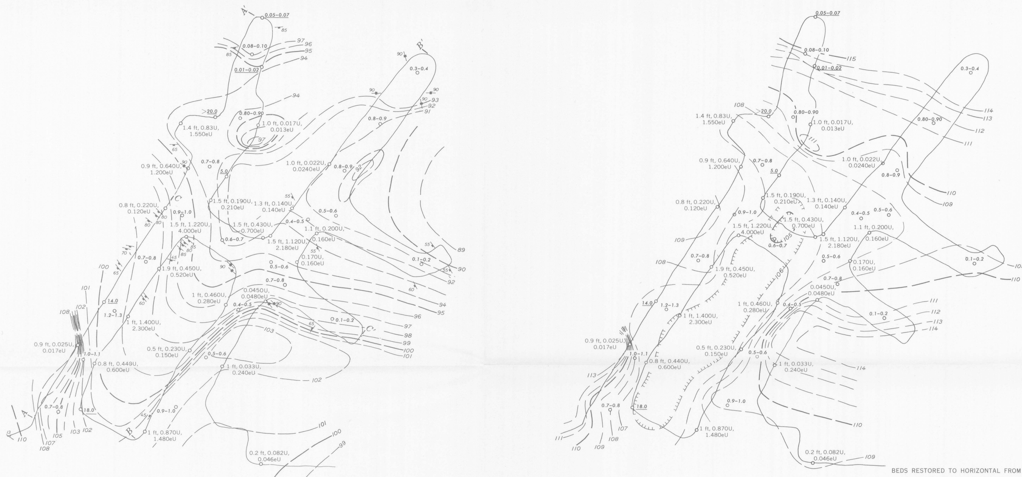
STRUCTURE CONTOURS DRAWN ON BASE OF THE SHINARUMP MEMBER OF THE CHINLE FORMATION AND PERCENTAGE OF URANIUM IN SAMPLES COLLECTED FROM BASAL BED OF SHINARUMP
