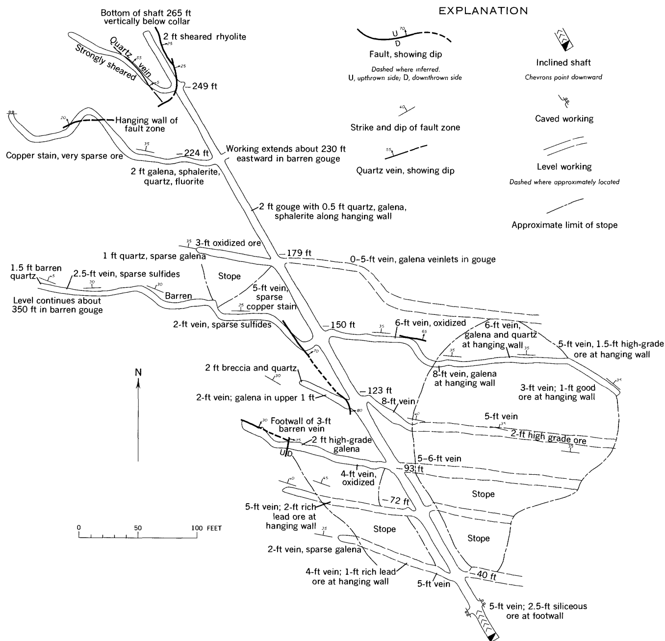
FIGURE 37.—Geologic map of the inclined shaft workings of the new Sinn Fein mine.
