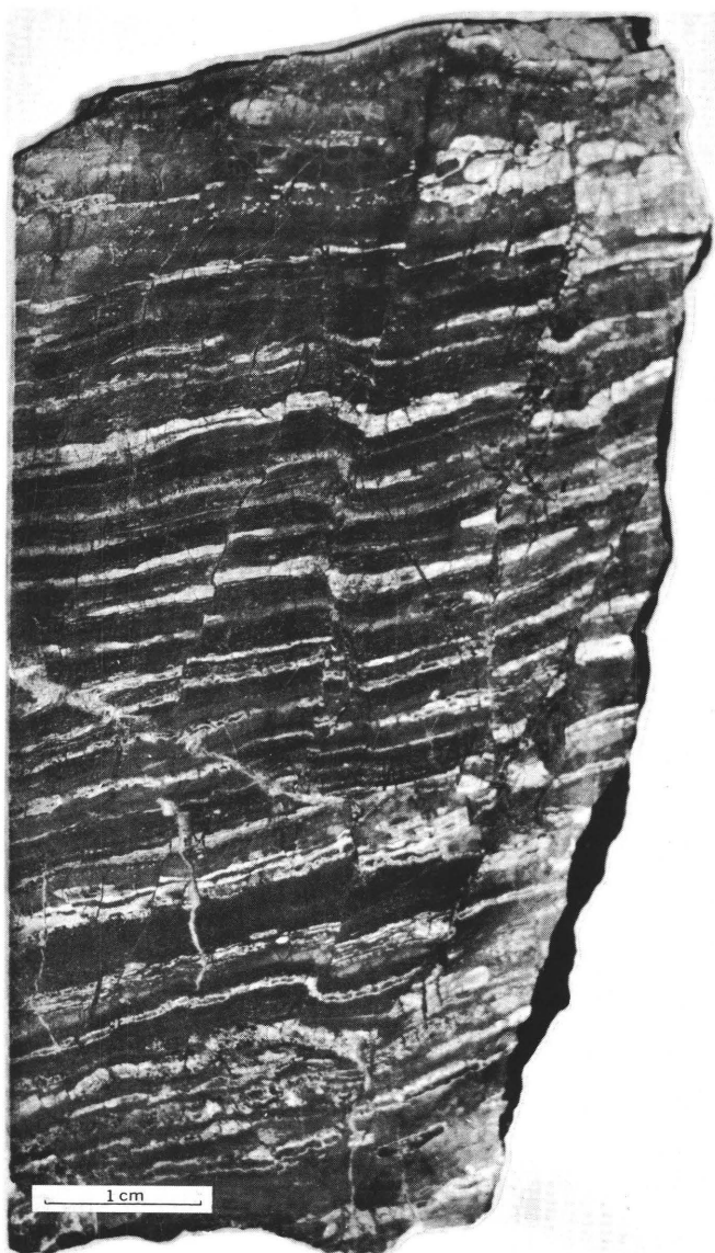
FIGURE 49.—Photograph of polished and etched slab of barite with interbedded chert, Hilltop barite mine deposit. Light-colored beds are chert, whitened by hydrofluoric acid.
