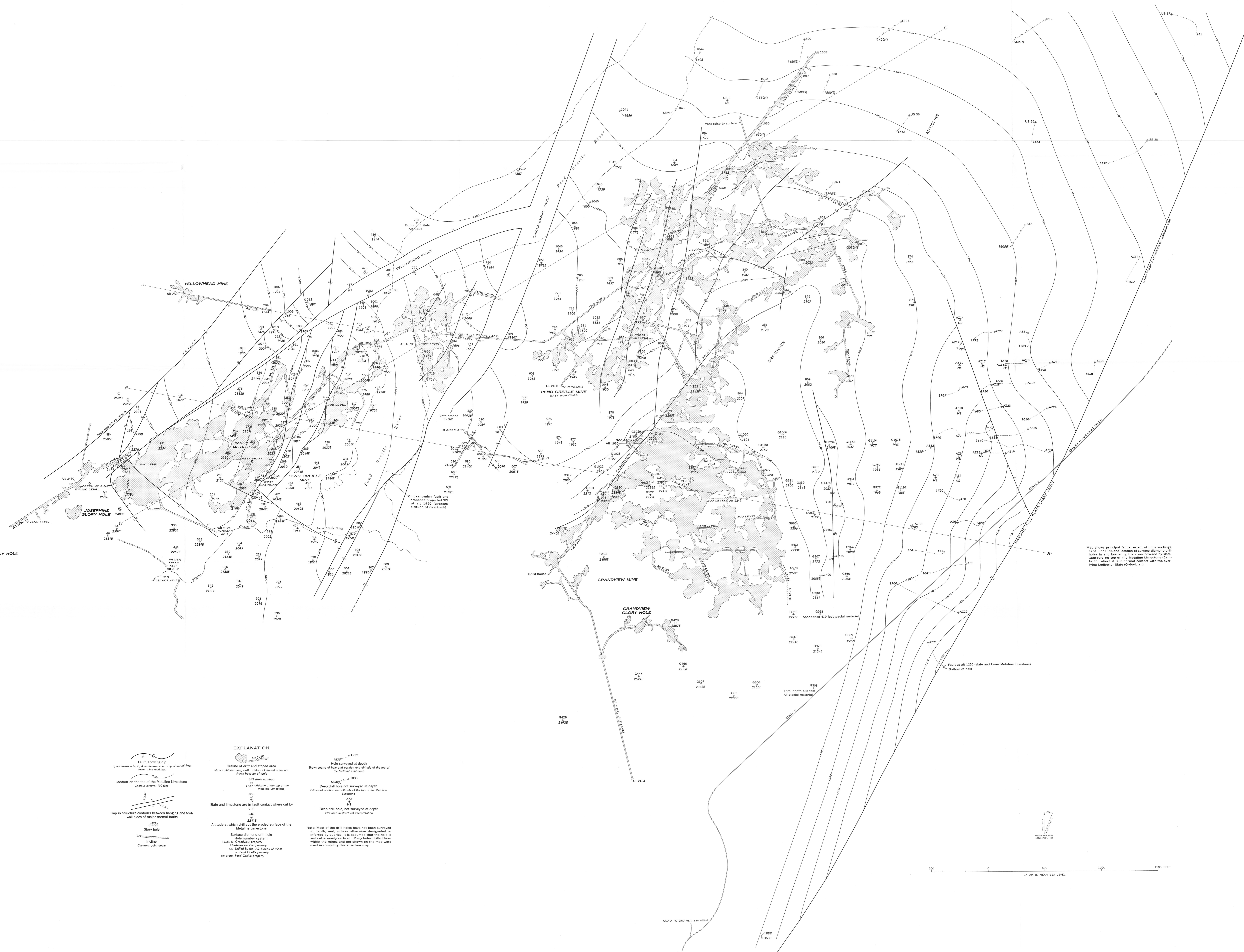
STRUCTURE CONTOUR MAP OF THE PEND OREILLE AND GRANDVIEW MINES AREA, PEND OREILLE COUNTY, WASHINGTON, SHOWING PRINCIPAL FAULTS, EXTENT OF MINE WORKINGS, AND LOCATION OF SURFACE DIAMOND DRILL HOLES
