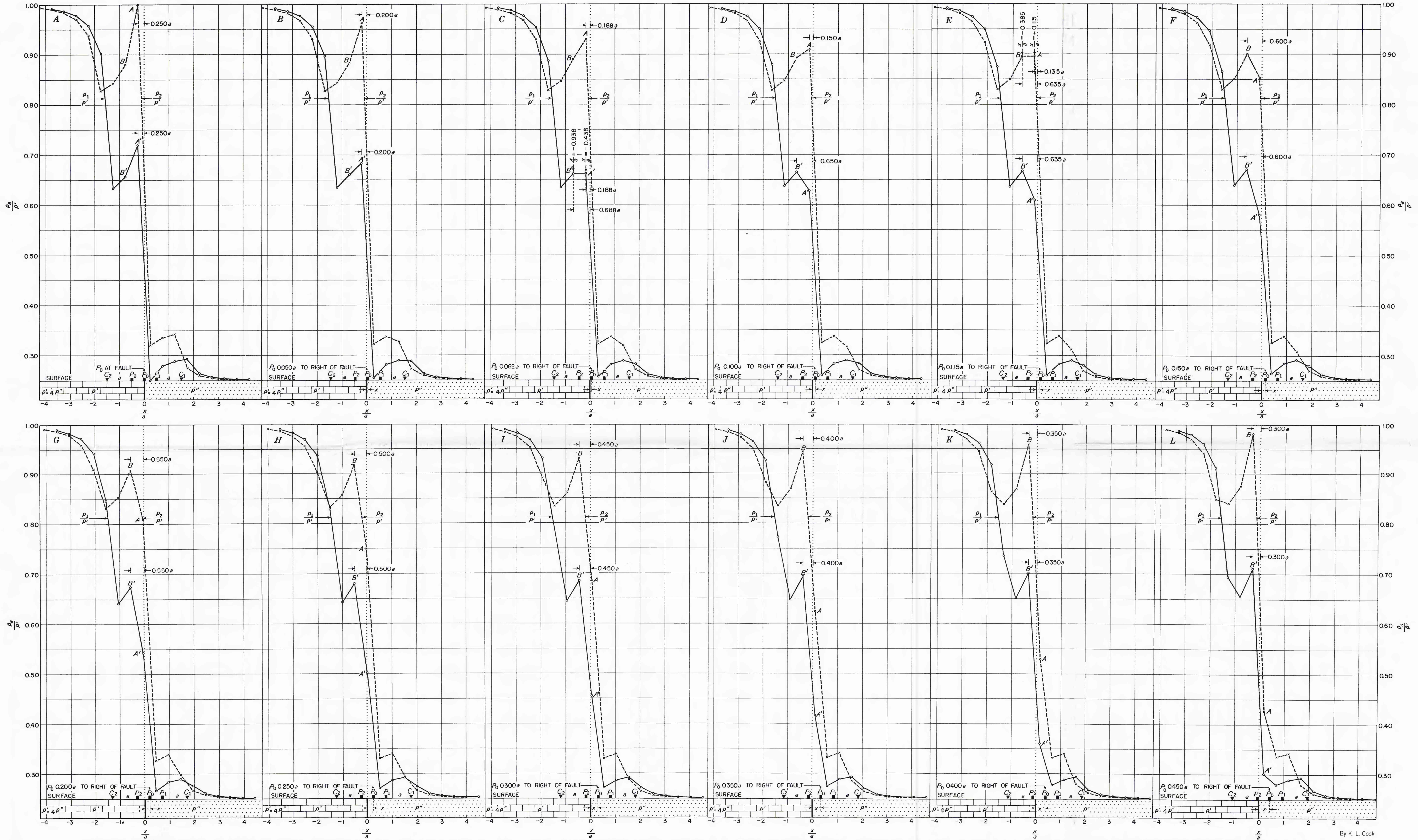
THEORETICAL FIELD PLOTS FOR HORIZONTAL RESISTIVITY PROFILES ACROSS VERTICAL FAULT, SHOWING DEPENDENCE OF SHAPE OF CURVES ON POSITION OF ELECTRODES RELATIVE TO FAULT, LEE CONFIGURATION (OFFSET PLOTTING)
