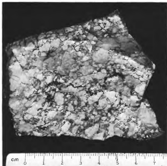
FIGURE 19.—Specimen from East Netta mine, showing "headcheese" texture that characterizes secondary chert formed by replacement of limestone in Joplin Member of Boone Formation during period of extensive leaching by ground waters. Some units, including the darker ones, are fragments of the earlier generation of chert.
