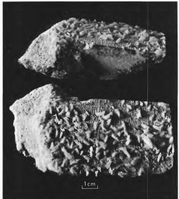
FIGURE 39.—Specimen showing "ripple marks" on jasperoid surface on floor of vug, with pink spar crystals projecting above the surface. From Pelican mine. Upper figure is mirror image of lower, to show cross section.
