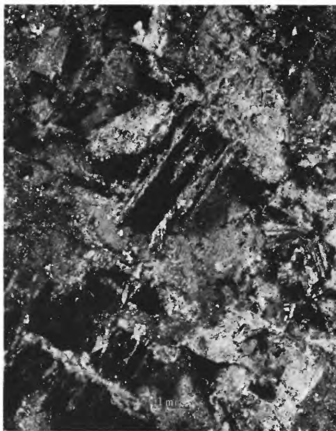
B. Leached galena showing thin residual plates mostly parallel to cleavage, but some in cube diagonal position; from Barr mine.
