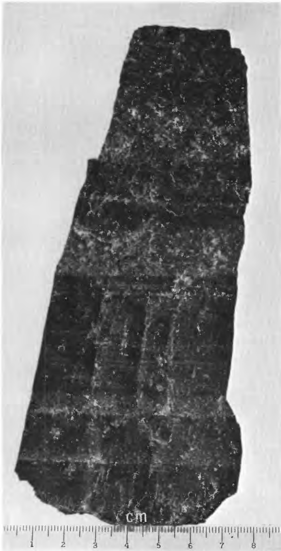
FIGURE 38.—Specimen from Wilson mine showing fine banding in jasperoid.
