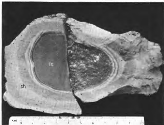
FIGURE 18.—Concentric banding in chert (ch) surrounding a nodular-shaped core of limestone (ls), from K bed, Mary Jane mine. Left side of specimen is sawed; right side shows natural break.
