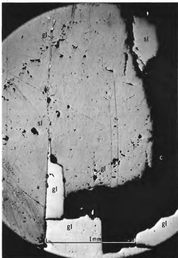
C. Polished section showing thin films left by leaching of galena, which are imbedded in a later crystal of sphalerite; from Midas mine. The film on left was originally at the cube surface of a galena crystal, of which only a small sector bordering the corrosion cavity is here shown. Galena, gl; sphalerite, sl; cavity, c.
