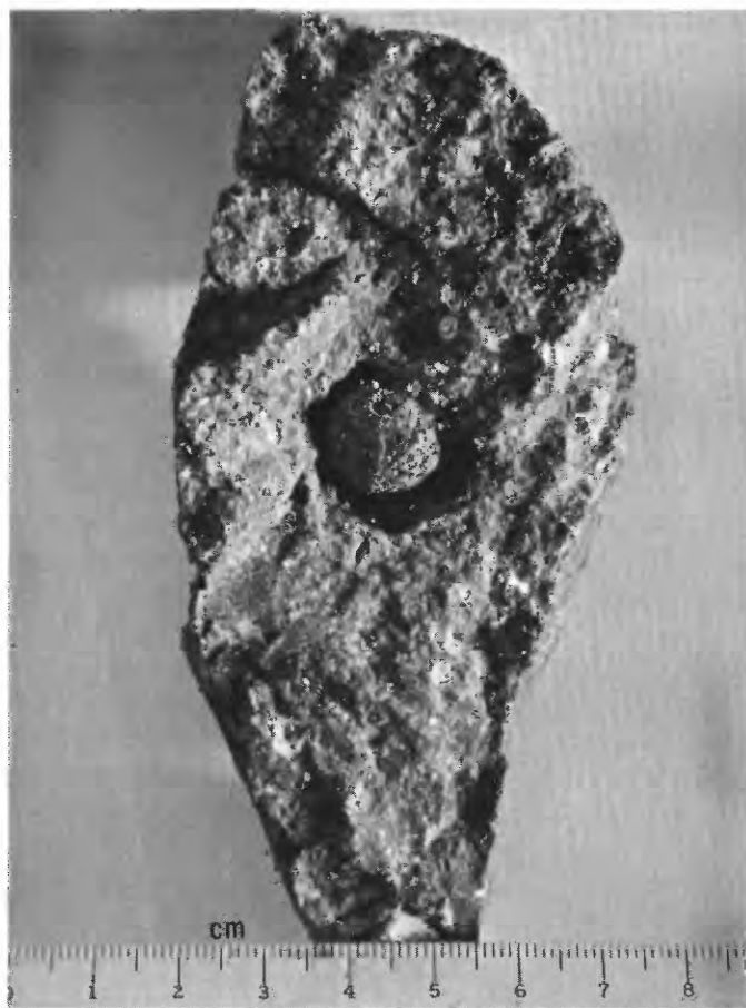
A. Cast of leached galena crystal in jasperoid, the cast containing a globular remnant of corroded galena hanging from the roof and later crystals of ruby jack (not visible in the photograph); from Lucky Syndicate mine.
