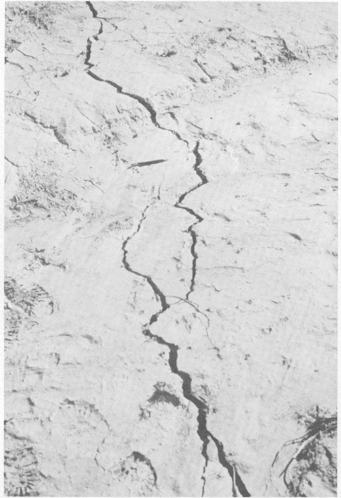
FIGURE 50. — October 1969. Sharp-edged fracture (fig. 49, e) that formed after the channel that it crosses carried water in September 1969. Pencil is parallel to the direction of net movement.
