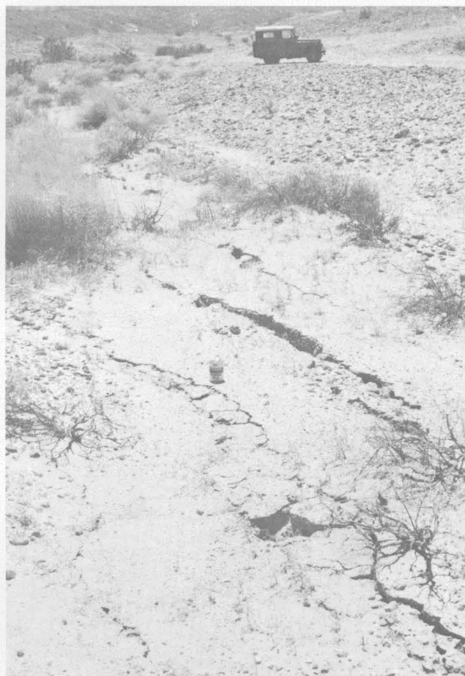
FIGURE 34.— Fractures showing left-lateral displacement at location 17.5, northeast of the central break. The en echelon arrangement of these fractures is opposite that of right-lateral fractures of the main breaks; that is, individual fractures here are oriented about 30° counter-clockwise from the trend of this fracture zone. Vertical and left-lateral displacements are about equal (40–50 mm).
