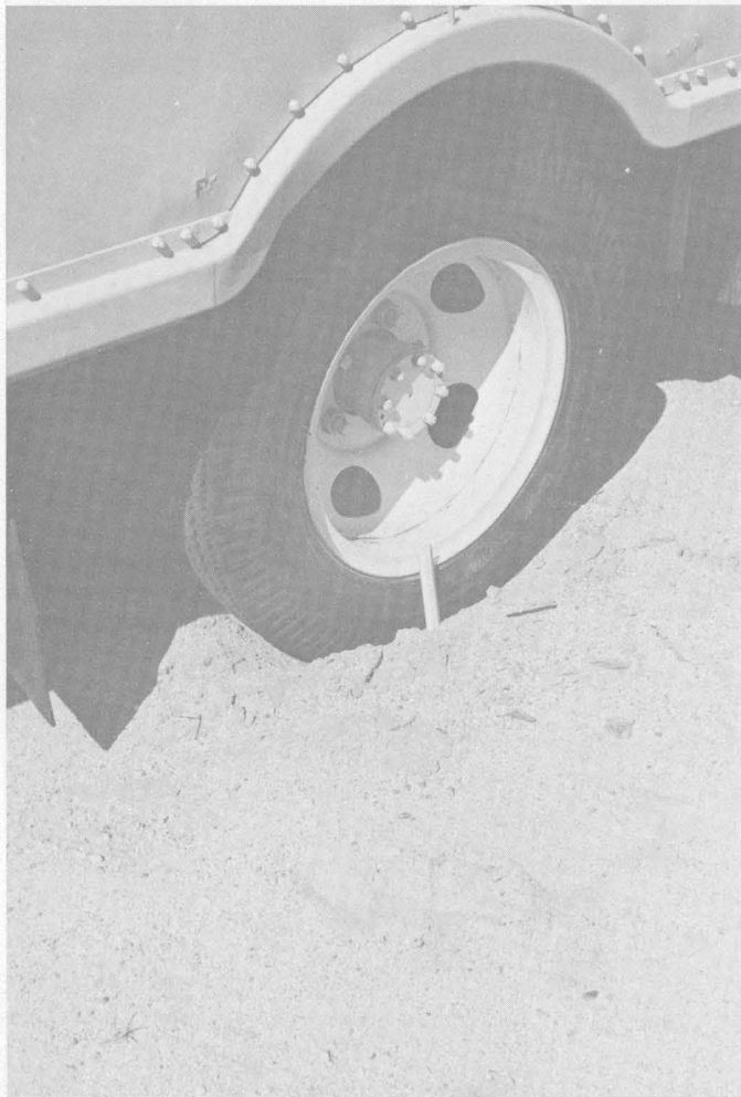
FIGURE 129. — Light truck that sank several centimeters into the dry desert sand, owing to vibratory ground motion, about 1.5 km southeast of Ocotillo Wells.
