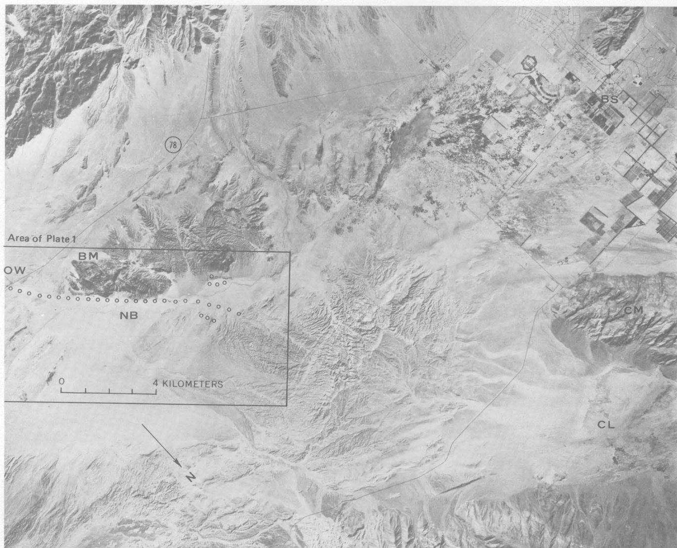
surface ruptures are shown as rows of open circles. BM, Borrego Mountain; BS, Borrego Springs; CB, central break; CL, Clark can be identified from plate 1. USGS aerial photographs USAF 665V 037 and 039, taken by U.S. Air Force, November 1967.
