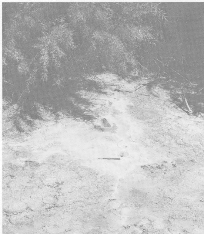
FIGURE 118.— Sand boils in late Quaternary lake-bottom deposits along the New River, about 55 km southeast of the epicenter.
