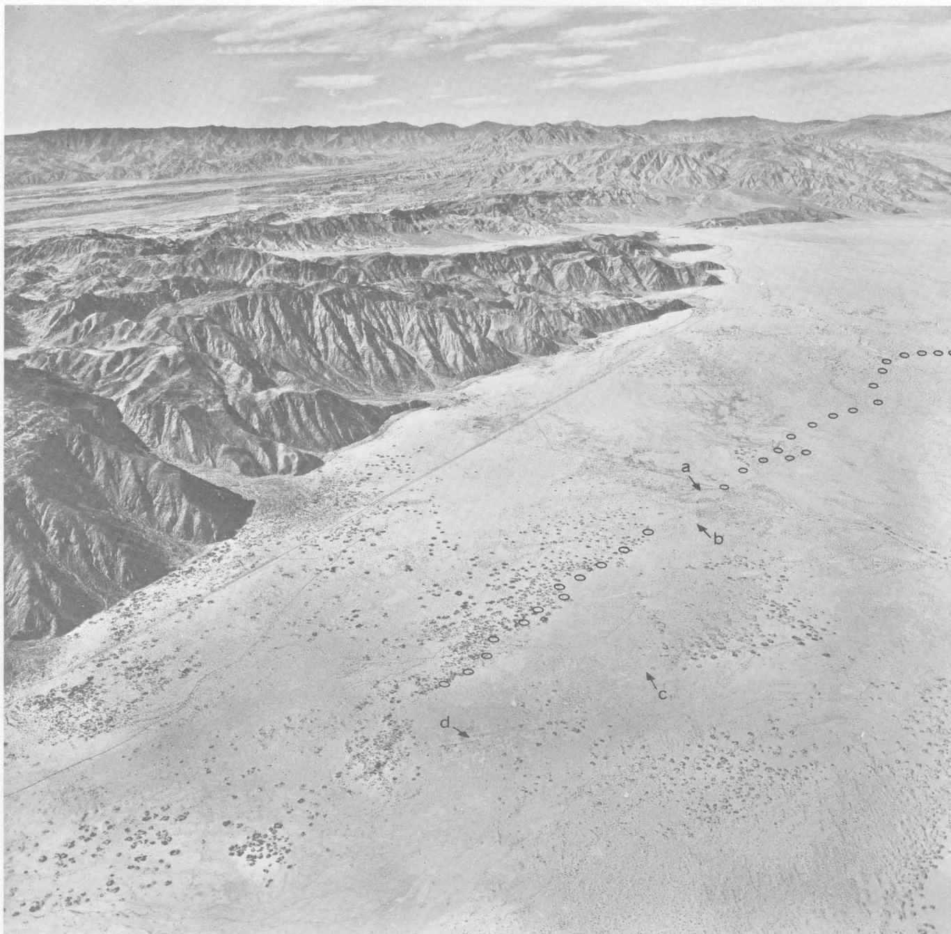
FIGURE 38. — View westward over south break (open circles) in November 1956. Mesquite-stabilized dunes are concentrated on the southwest side of the fault, which acts as a barrier to ground water. Relict collapse fissures visible as lines of bushes are at a , b , and d . A prominent collapse fissure developed later (but before the 1968 earthquake) at c . (See Clark, "Collapse Fissures Along the Coyote Creek Fault," this volume.) U.S. Geological Survey photograph OAJ 5-129, November 1956.
