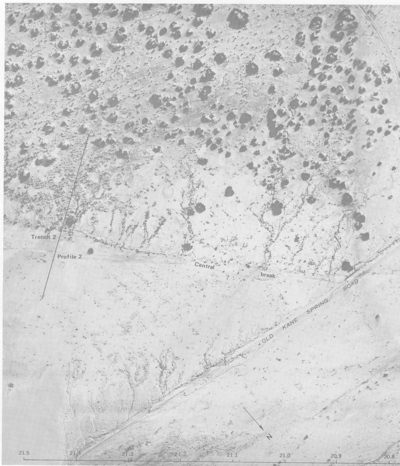
FIGURE 80.—Vertical aerial photographs of central and branching breaks of the 1968 earthquake at Old Kane Spring Road showing a shallow graben between the breaks and the location of trenches 1, 2, and 4 and profiles 1 and 2. (These photographs were taken in April 1969, about 1 year after the earthquake. Fig. 37 shows the same area a few weeks after the earthquake and gives a general
