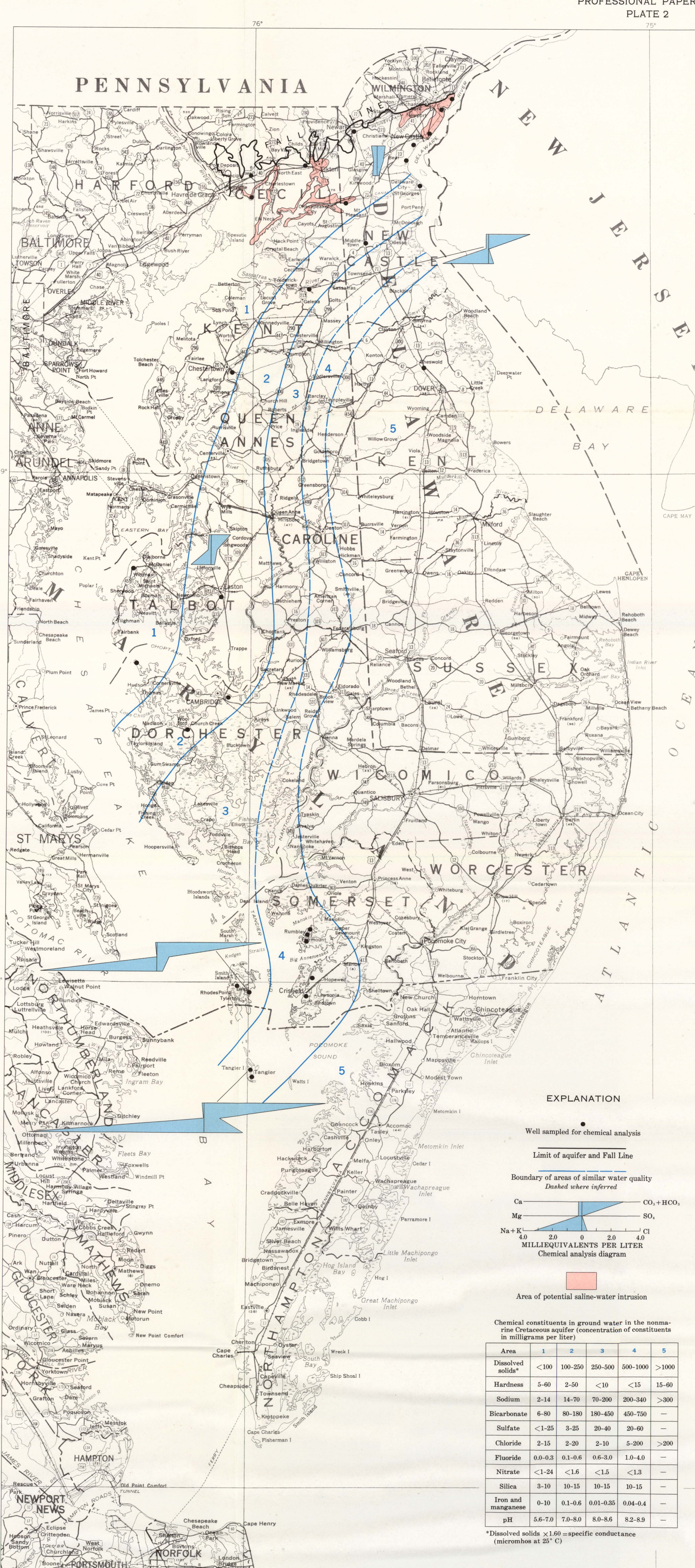
CHEMICAL QUALITY OF GROUND WATER AND AREA OF POTENTIAL SALINE-WATER INTRUSION IN THE NONMARINE CRETACEOUS AQUIFER
