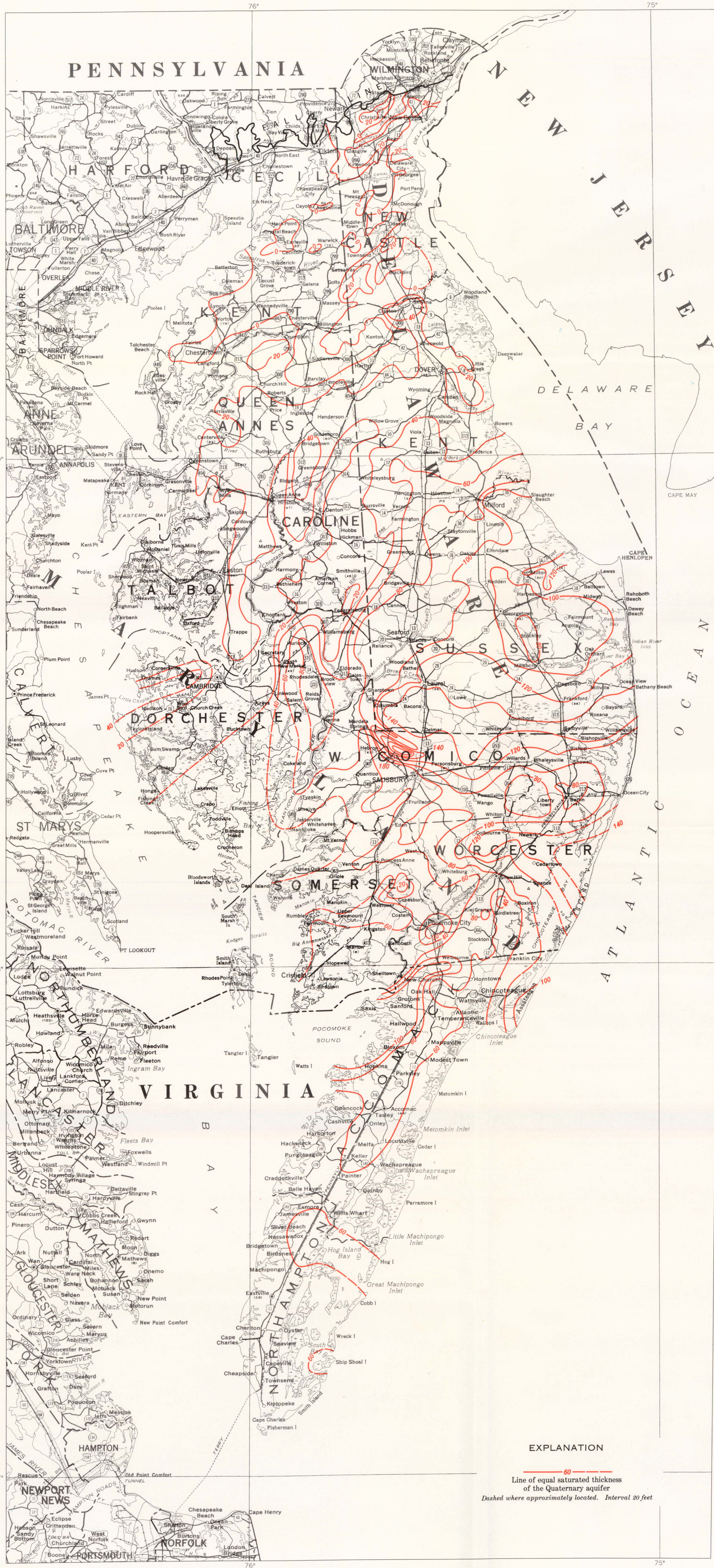
SATURATED THICKNESS OF THE QUATERNARY AQUIFER
